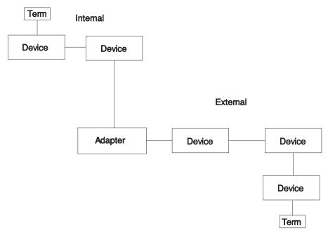
Figure B-2. SCSI Chain with Internal and External Devices
