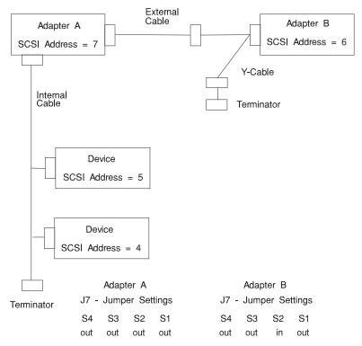
Figure B-3. Adapters Sharing Internal Devices
