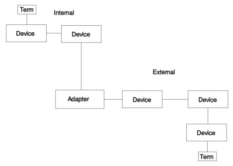
Figure A-1. SCSI Chain with Internal and External Devices
