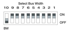
Figure C-5. Bus Width Switch Position
