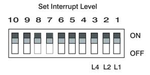
Figure C-1. Interrupt Level Switch Positions
