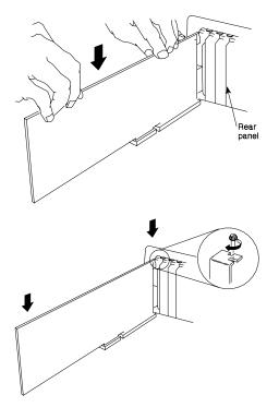
Figure 2-2. Inserting the X.25 Adapter Into the Expansion Slot
