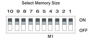
Figure C-2. Memory Size Switch Position
