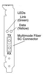
Figure 3. LEDs on the Gigabit Ethernet-SX PCI Adapter
