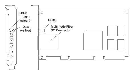
Figure 1. The Gigabit-SX PCI Adapter
