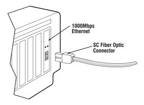
Figure 2. Connecting the Adapter to the Network
