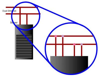
On the storage side, the following diagrams all depict duplicated, direct connections between the cluster nodes and shared storage. In practice, with the use of SANs and (optionally) the IBM SAN Volume Controller, redundant connections between each cluster node and each SAN fabric would be needed to avoid SPOFs in the node to storage connections.
