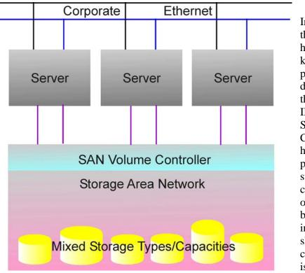
In pSeries lingo, all the server sees is an hdisk – it doesn't know (or care) what physical storage device is providing that disk resource. IBM's TotalStorage SAN Volume Controller (SVC) is a hardware/software product that adds this storage virtualization capability. While it is optional when building an IT infrastructure, it should be strongly considered when there is a need for an
