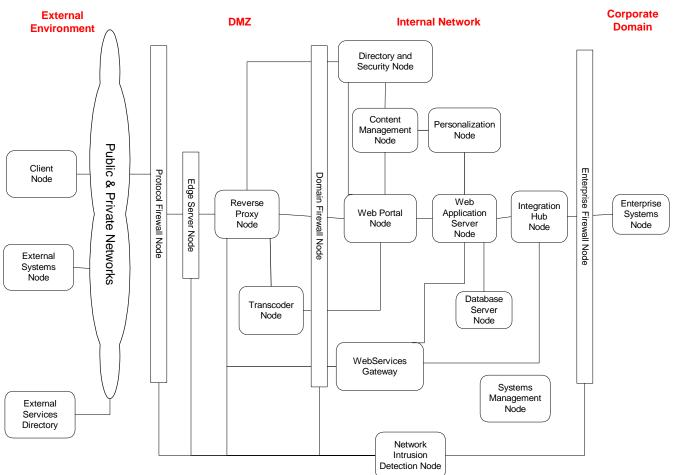
Figure 2 - Conceptual-level System Topology Diagram
