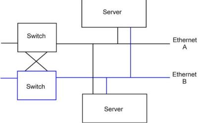
A further note about the server Ethernet connections: many Ethernet adapters now offer dual ports on a single adapter. Keeping the example diagram in mind, it is tempting to use one port on a single adapter for Ethernet A, while the second port is connected to Ethernet B. Be aware that this approach makes the
