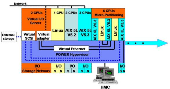
Figure 7 - System p5 Advanced POWER Virtualization Diagram
