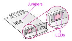
If the interface card fails to establish a network link through autonegotiation, you might need to change the position of configuration jumpers P1, P2, and P3 on the interface card (see the figure on the next page). The default position is P1 AUTO=ON. In this position, the interface card attempts to connect automatically to the network at the detected speed (10 or 100 Mbps) and communication mode (full-duplex or half-duplex). The options are:
