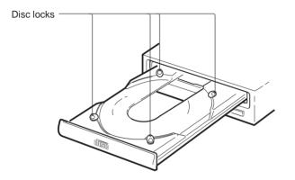
**4** Gently push the drawer or press the eject button to close the drawer. The drive may begin reading the Table of Contents (TOC) data when it accepts the disc. The busy indicator lights up in amber while the drive is reading the TOC.
