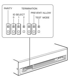
The recommended jumper for use is AMP Shunts (14227-1), JAE Short Socket (PS-2SH4-1) or equivalent.
