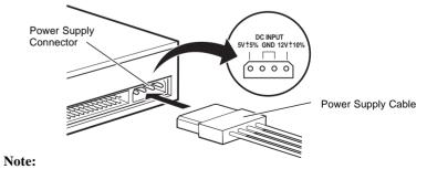
The power supply connector is designed to fit only in one way. Do not attempt to force the cable in upside down, otherwise the CD-ROM drive will be damaged and the product warranty void.
