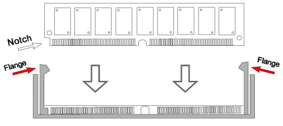
Figure 1-1 Inserting a SIMM module
