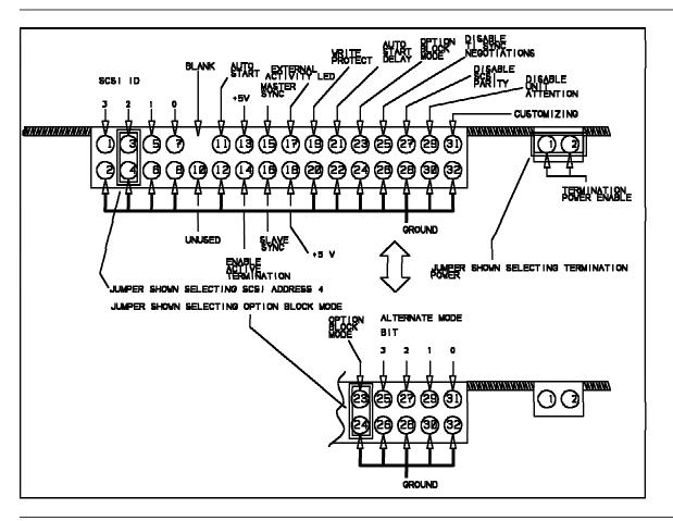
. Figure 31. 68 pin Single Ended Front Option Jumper Block (& TermPower Block)
