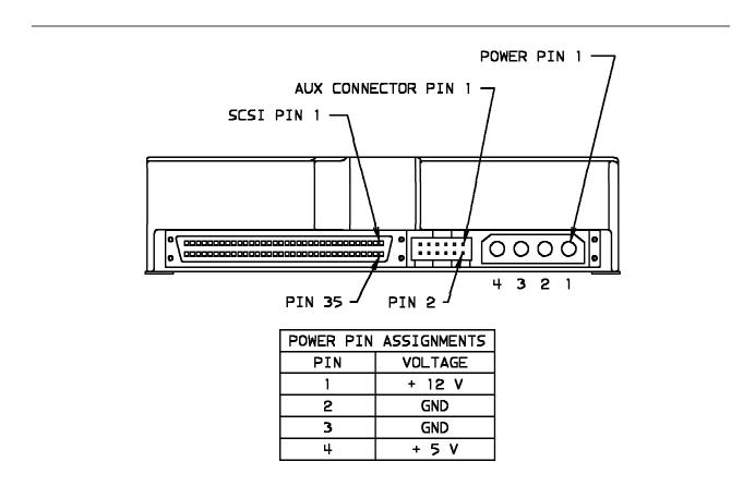
Figure 27. Electrical connectors (rear view) -- 68 pin models.
