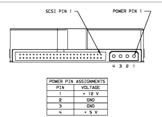
Figure 28. Electrical connectors (rear view) -- 50 pin models.
