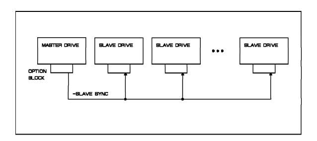
Figure 38. Daisy-Chain Connection of Synchronization Bus
