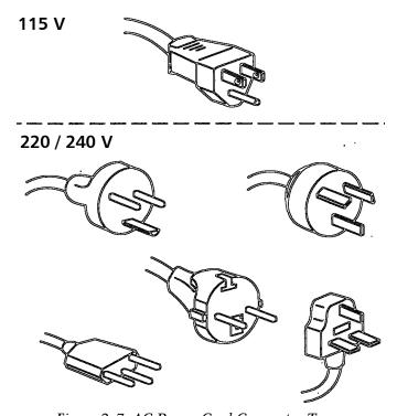
Figure 2-7 AC Power Cord Connector Types
