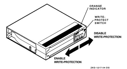
Figure D-5 Write-Protect Switch on Tape Cartridge
