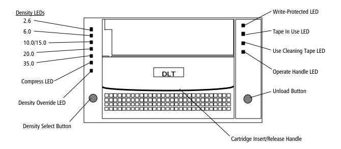
Figure 2-8 DLT 7000 Front Panel
