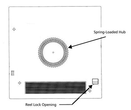
5. Look at the bottom of the tape cartridge, holding it as shown in Figure D-2.
