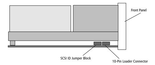
Figure 2–5 Loader Connector Block Location (Rackmount Version Shown)
