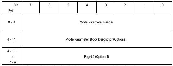
Figure 5-33 MODE SELECT Mode Parameter List - Data Format
