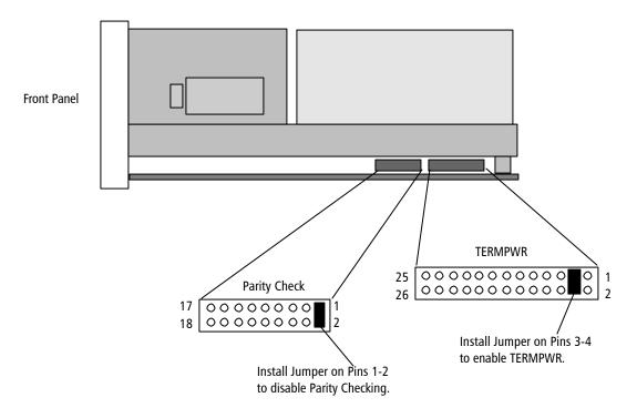
Figure 2-2 DLT 7000 TERMPWR and Parity Check Jumper Locations (Rackmount Version Shown)
