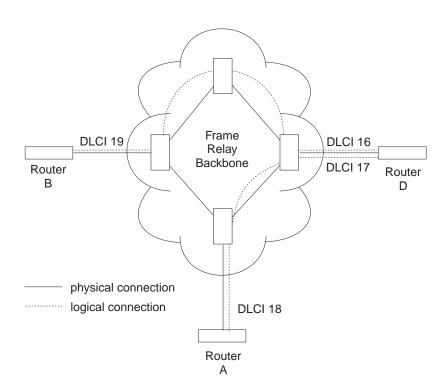
Figure 21. DLCIs in Frame Relay Network
