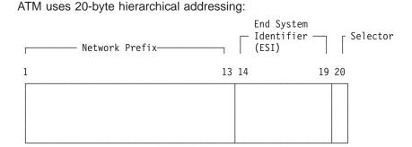
The first 13 octets of an ATM address are the Network Prefix. Each switch in your ATM network must have a unique Network Prefix. ATM switches use the Network Prefix to route VCC setup requests the destination ATM switch. End systems, like this router, retrieve their Network Prefix from their ATM switch when they activate.
