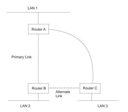
If the primary link between routers A and B fails, WAN reroute establishes an alternate link between routers B and C. Routers A and B can then communicate through router C.
