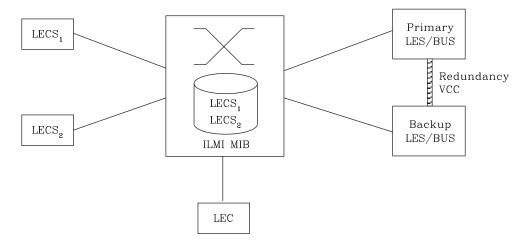
Figure 17. LAN Emulation Redundancy
