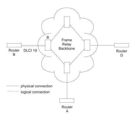
Figure 22. DLCIs in Frame Relay Network
