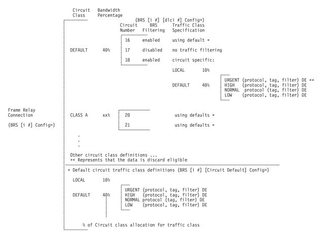
**Note:** All protocols are initially assigned to the NORMAL priority queue of the DEFAULT traffic class. You can assign a protocol, filter, or tag to any priority queue within a traffic class.
