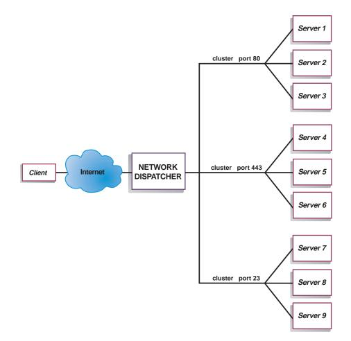
Figure 42. Example of Network Dispatcher Configured with 3 Clusters and 3 Ports
