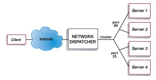
Figure 40. Example of Network Dispatcher Configured With a Single Cluster and 2 Ports
