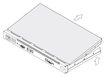
Figure A-2. Removing the Cover
