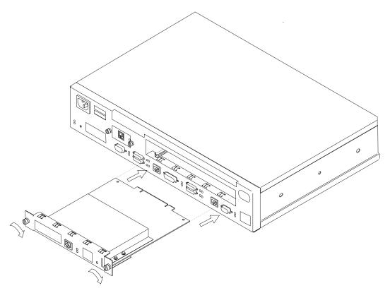
Figure A-5. Installing the Optional Adapter (Actual adapter may appear different.)
