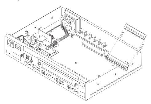
Figure A-11. Installing the Flash SIMM (14T and 24x Models)
