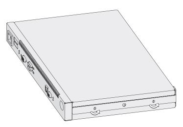
Figure 1-2. Removing the Screws on the Mounting Bracket
