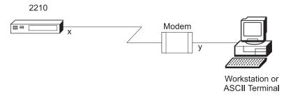
Figure 3-2. Remote Connection to 14.4 Kbps Modem Port Feature (14T and 24x Models)
