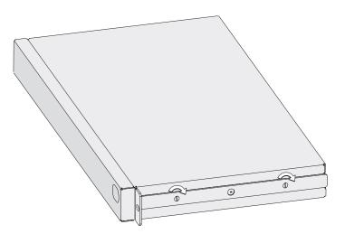
Figure A-4. Replacing the Screws and Mounting Bracket
