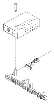
Figure A-8. Installing the 14.4 Kbps Modem Port Feature
