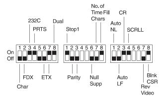
Figure 3-5. Setup Attributes for the IBM 3101 Display Terminal
