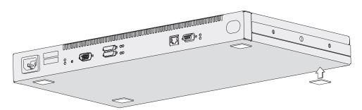
Figure 1-1. Attaching the Feet to the Bottom of the IBM 2210
