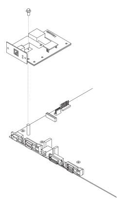
Figure A-7. Installing the EIA 232 Service Port Feature
