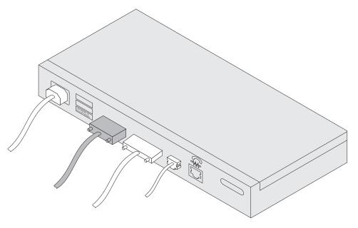
Figure 3-4. Attaching an ASCII Terminal to the Service Port
