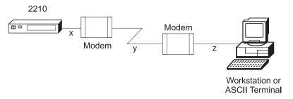
Figure 3-3. Remote Terminal Connection to the Primary or Secondary EIA-232 Service
