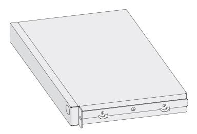
Figure A-1. Removing the Side Screws
