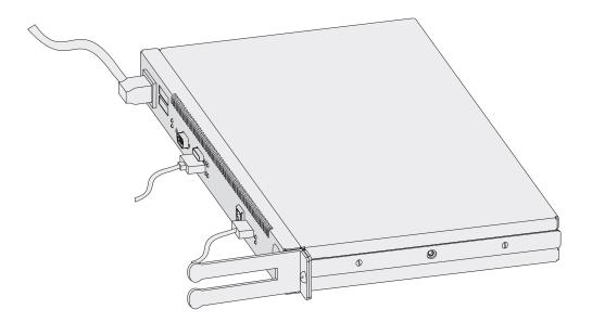
Figure 1-17. Connecting the Power Cord to the IBM 2210
