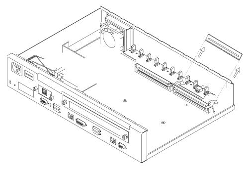
Figure A-10. Removing the Flash SIMM (14T and 24x Models)
