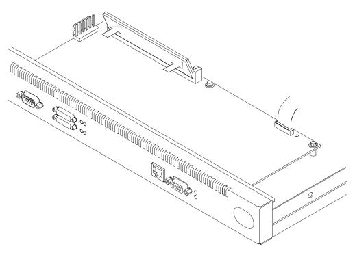
Figure A-9. Replacing the DRAM SIMM in 12x Models
