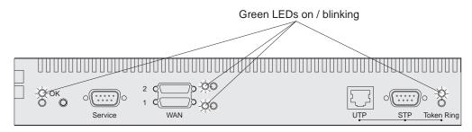
Figure 1-18. LEDs On or Blinking on Port Side after Successful Boot
