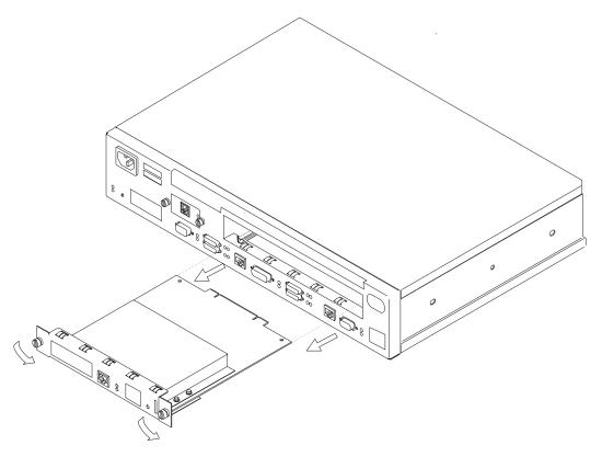
Figure A-6. Removing the Adapter (Actual adapter may appear different.)
