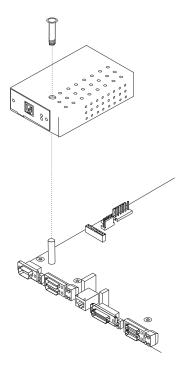
Figure 4-42. Installing the 14.4 Kbps Modem Port Feature
