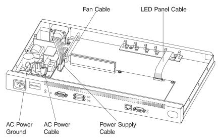
Figure 1-17. View of Cable Connections (12x Models)
