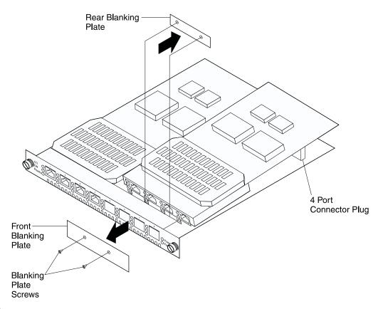
Figure 4-43. Installing the 4 Port Dial Access Modem Card
