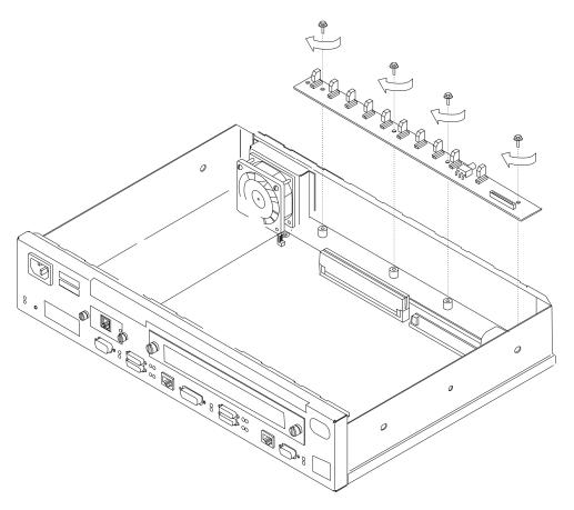
Figure 4-36. Replacing the LED Panel (14T and 24x Models)
