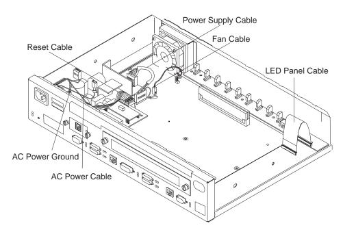
Figure 1-18. View of Cable Connections (24x Models)
