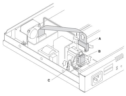
Figure 4-23. Connections to the Power Supply (12x Models)
