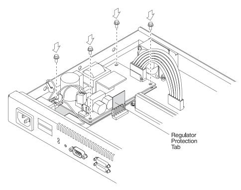
Figure 4-25. Replacing the Corner Screws (12x Models)
