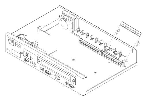
Figure 4-21. Removing the Flash SIMM (14T and 24x Models)
