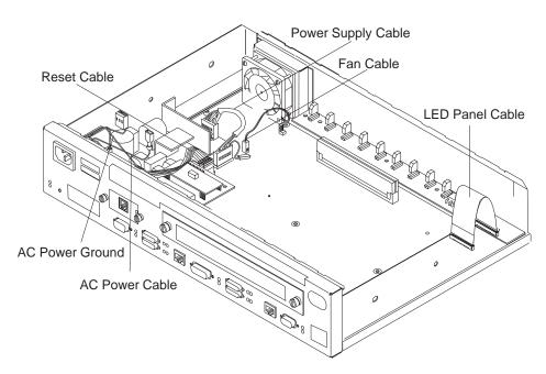
Figure 4-28. Connections to the Power Supply (14T and 24x Models)
