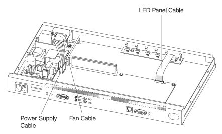
Figure 4-5. Cables Attached to the System Board (12x Models)
