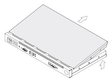
Figure 4-2. Removing the Cover
