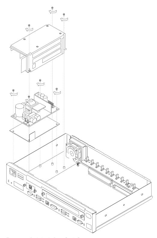
Figure 4-30. Replacing the Power Supply Cover
