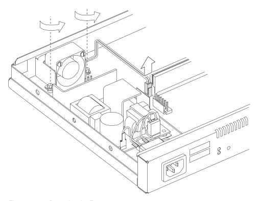
Figure 4-31. Removing the Fan
