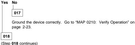
Is the RS 232 cable between the terminal and the IBM 2210 grounded correctly and shielded?
