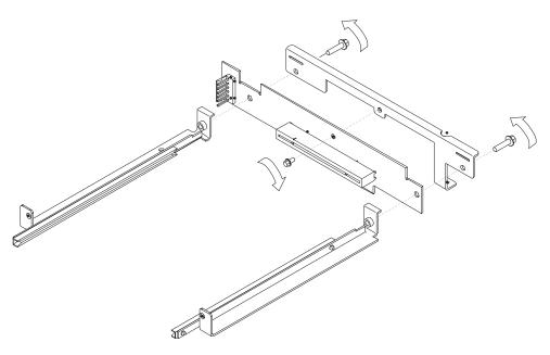
Figure 4-37. Assembling the Riser Card Assembly
