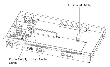
Figure 4-11. Attach Cables to the System Board (12x Models)
