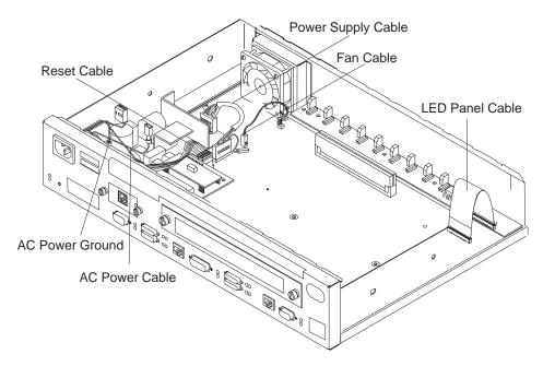
Figure 4-29. Connections to the Power Supply (14T and 24x Models)
