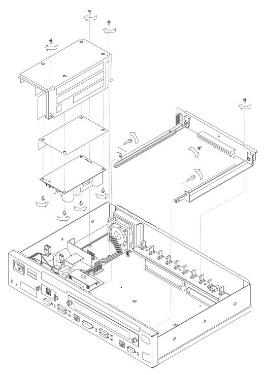
Figure 4-38. Installing the Adapter Enablement Feature
