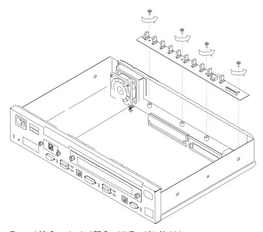
Figure 4-35. Removing the LED Panel (14T and 24x Models)
