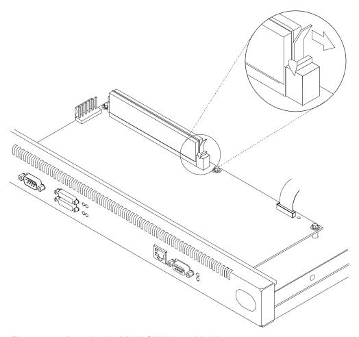
Figure 4-19. Removing the DRAM SIMM in 12x Models
