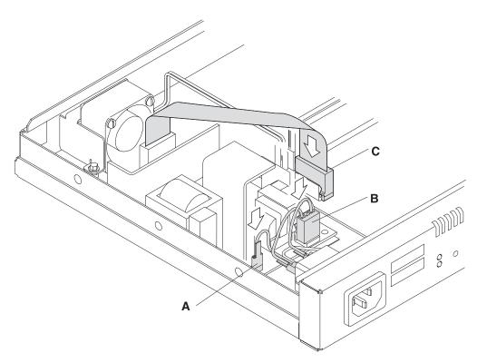
Figure 4-26. Connections to the Power Supply (12x Models)
