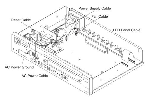
Figure 4-12. Cables Attached to the System Board - 14T Model
