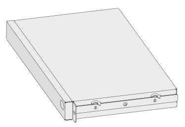
Figure 4-4. Replacing the Screws and Mounting Bracket
