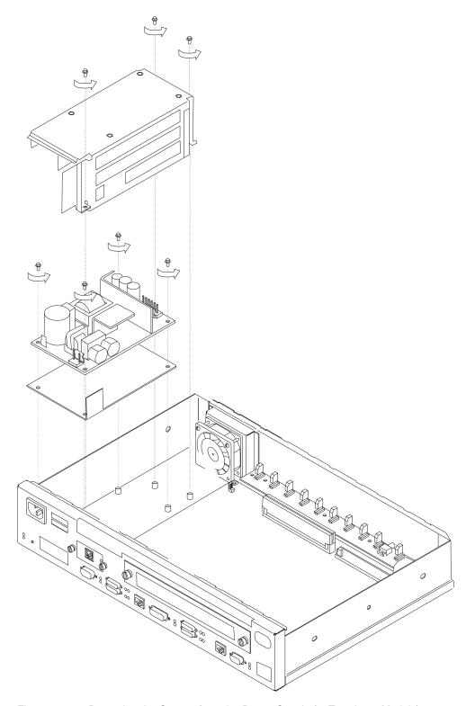
Figure 4-27. Removing the Screws from the Power Supply (14T and 24x Models)
