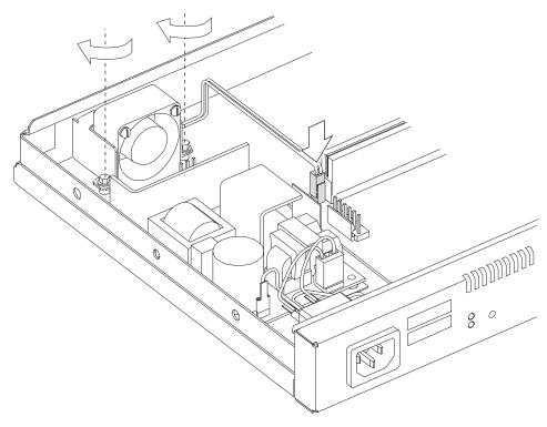
Figure 4-32. Replacing the Fan
