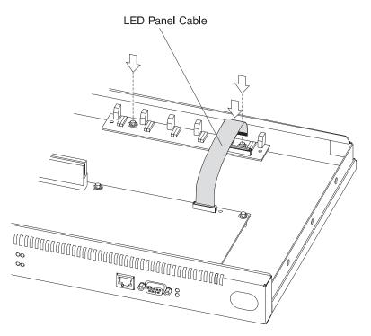
Figure 4-34. Replacing the LED Panel (12x Models)
