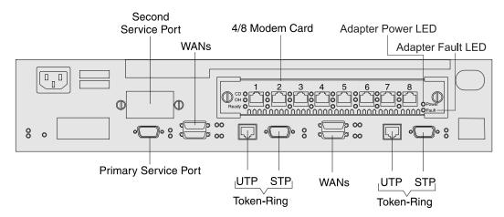
Figure 1-11. Model 24M with the 4 Port Dial Access Modem Card Installed
