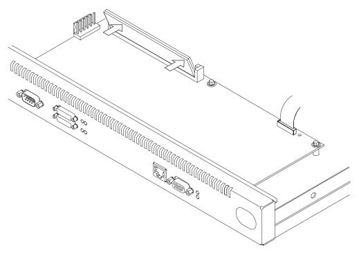
Figure 4-20. Replacing the DRAM SIMM in 12x Models
