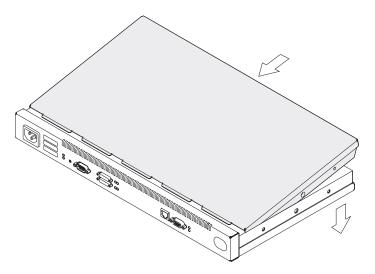
Figure 4-3. Replacing the Cover
