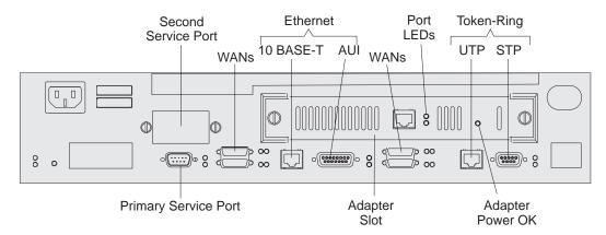
Figure 1-10. Model 24M with an Optional Adapter Installed
