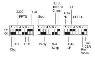
Figure A-1. Setup Attributes for the IBM 3101 Display Terminal
