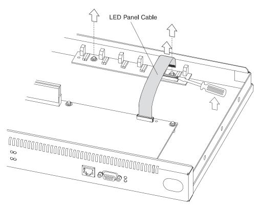
Figure 4-33. Removing the LED Panel (12x Models)
