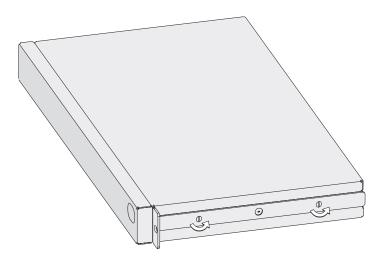
Figure 4-1. Removing the Side Screws
