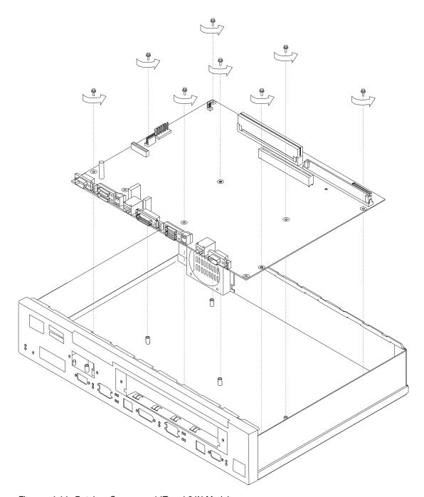
Figure 4-14. Retainer Screws on 14T and 24X Models
