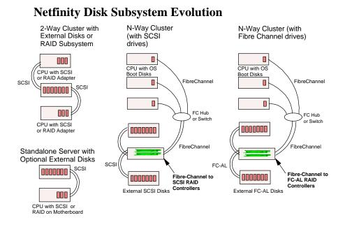
Prior to 1997, customer solutions were based primarily on standalone servers with internal SCSI disks and/or a single, nearby SCSI storage expansion enclosure. Then the introduction of the IBM EXP10 in November 1997 made 2-way clustering possible, allowing two servers to share external storage devices.
