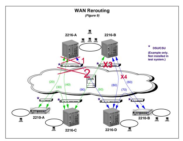
Following is an overview of the different WAN failure scenarios that were tested.
