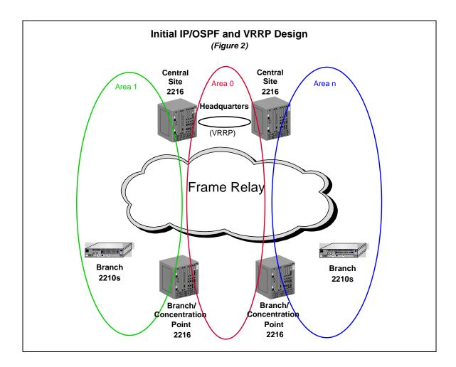
In order to achieve the required availability, the fast converging OSPF routing protocol was the obvious choice. To limit the size of routing tables and OSPF flows, a network of this size requires multiple areas and address summarization. Per the above logical diagram:
