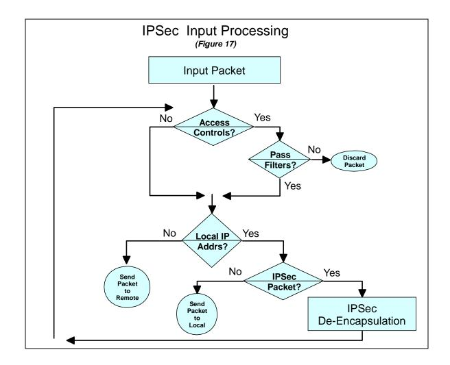
Only the second test, "*Pass Filters*?", actually involves the Access Controls filters. All input traffic on a port undergoes one or both of the last two tests. This means that all IPSec processing will take place for local resources and that IPSec packets destined for remote resources will be forwarded **even if Access Controls are not enabled for the interface**. The significance of any security exposures caused by the lack of this extra filtering is debatable.
