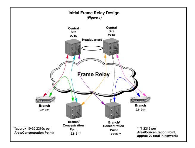
The new network will center around a pair of headquarter based 2216 M400 routers (hereafter also referred to as the *Central Site* routers) connected locally by a token ring segment. Also attached to that ring will be the FEPs/mainframes and servers accessed by remote site 2210 and 2216 routers. The remote sites will be organized into areas each containing 10 to 20 2210 Branch Office routers. The 2210s are each connected via Frame Relay PVCs (shown in the above figure by the colored lines) to:
