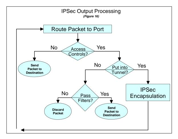
If a port's output filters are enabled, prior to a packet's transmission it is checked against the output filter rules for that port. Packets are identified for placement into a specific IPSec tunnel based on matches on IP addresses and/or protocols as specified by the filter's entries.
