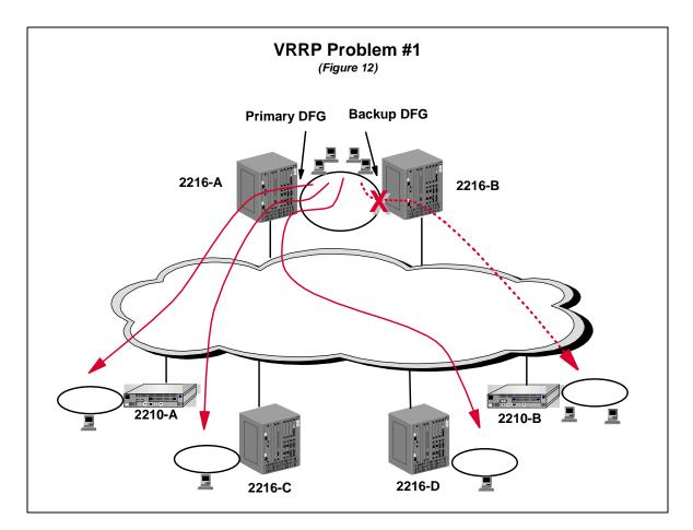
As shown in *Figure 12*, even though 2216-A's token ring port's IP address was the DFG for all the work stations on the Central Site ring, the pings to one of 2210-B's work stations (identified by the dotted line) were being sent to 2216-B's port thus causing the interruption of that traffic when that port was disabled. It's easier to understand what was happening if the problem scenario is overlaid on the Frame Relay components of the network as shown in Figure 13 on the next page.
