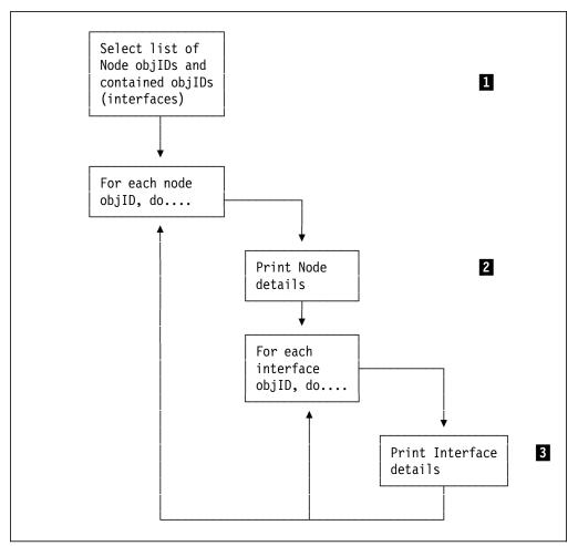
Figure 33. Logic for wtqnode Samples
