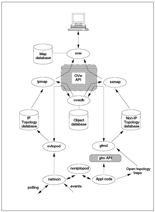
Figure 130. Components of IP and Open Topology
