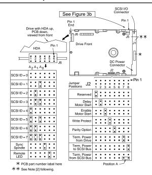
Figure 3a. Drive configuration for ST11200 family
