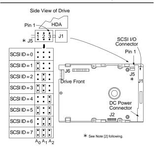
Figure 3b. Drive configuration for ST11200 family
