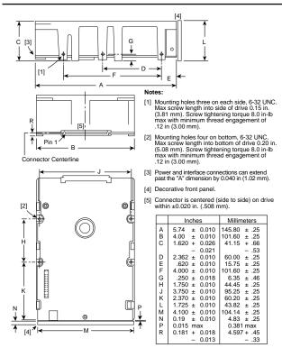
Figure 6. Mounting configuration details for ST11200NC model drives
