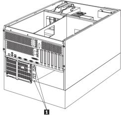
Remove the voltage regulator card mounting screws
