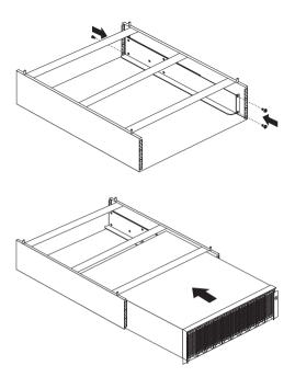
**Removing Cage Nuts:** Device installation might require the removal or moving of the rear-pane cage nuts. If you need to move the cage nuts, follow this procedure to move them and then go to "Installing Cage Nuts" on page 212 to install them in the correct position.
