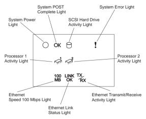
System Power Light: When this green light is lit, system power is present in the server. When this light flashes, the server is in standby mode (the system power supply is turned off and AC current is present). When this light is off, it indicates either power supply failure, an AC power failure, or a light failure.
