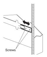
Insert screws (6M by 16 mm) through the mounting rail to the slide-bracket assembly. Do not tighten the screws.
