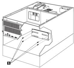
Remove the power backplane cover screws 1, then; remove the power backplane cover.
