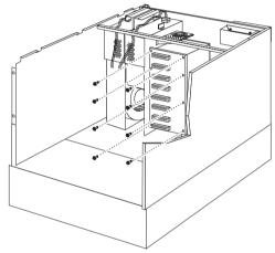
Remove the DASD backplane screws 1, then; remove the DASD backplane.
