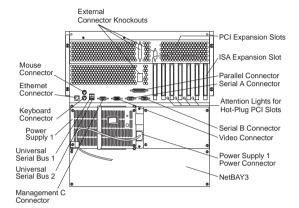
**Keyboard Connector:** The keyboard cable connects here.
