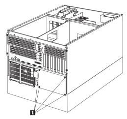
Remove the power supply filler plate screws 1, then; remove the power supply filler plate.
