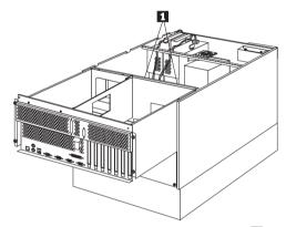
a. Remove the power backplane cover screws 1 .
