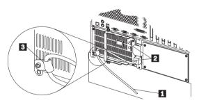
Plug the power cord into a properly grounded electrical outlet.
