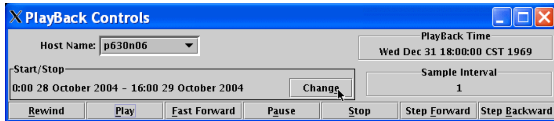
Figure 3-3 jtopas playback control panel
