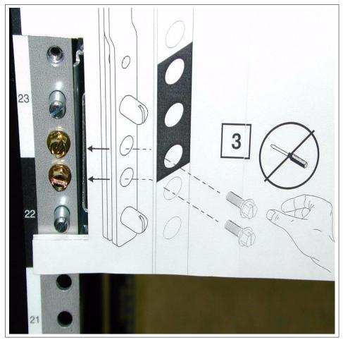
Figure 3-12 Slide mounting plate in position
