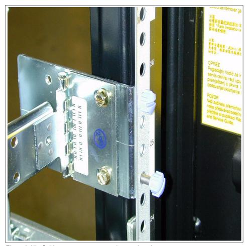
Figure 3-27 Cable management arm rack mounting plate
