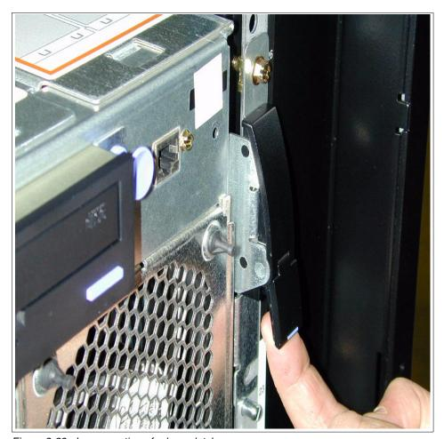
Figure 3-22 Lower section of release latch
