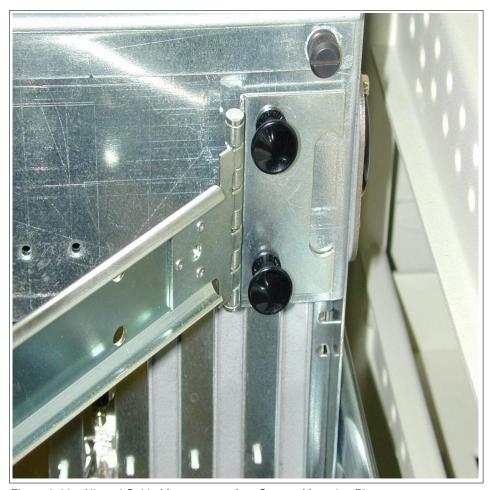
Figure 3-26 Aligned Cable Management Arm System Mounting Plate
