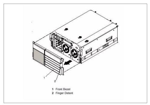
Figure 3-20 Front bezel removal.
