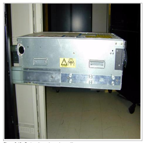
Figure 3-19 System drawer in service position
