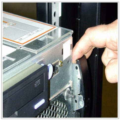
Figure 3-23 Top of release latch
