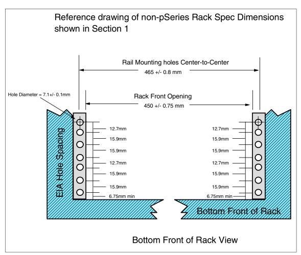
Figure 3-30 non-pSeries bottom front rack view
