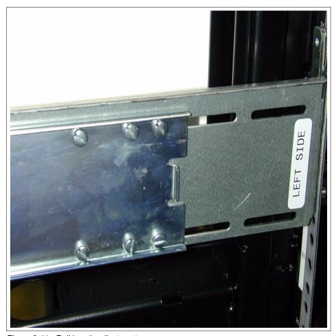
Figure 3-11 Rail length adjustment screws
