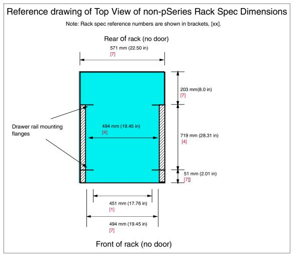
Figure 3-28 Reference drawing of non-pSeries rack dimensions
