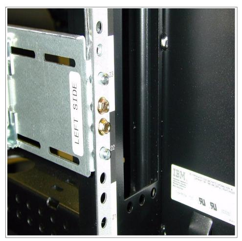
Figure 3-13 Rear rail pin in noted hole location
