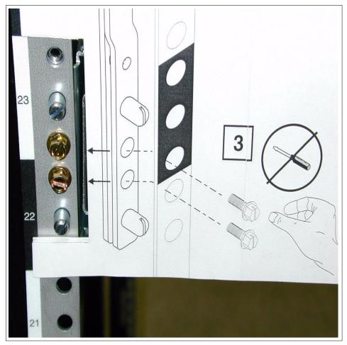
Figure 3-7 Slide mounting graphic (left side)
