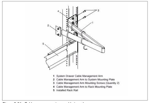
Figure 3-24 Cable management assembly in rack
