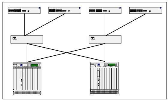
Figure 3-3 Star topology in an Ethernet network
