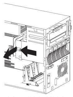
Release the fan assembly latch and slide the fan assembly out of the server.
