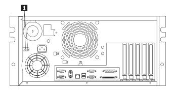
Power Supply Lights: These green LEDs indicate a power good status for each of the 175-watt modules in the power supply. If any power supply light is not illuminated when the Power-On Light on the front of the server is on, there is a problem with that power supply. The power supply shipped with the server has two lights, one for each module in
