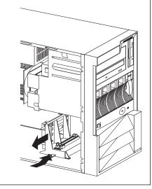
To remove a card support from a slot 1 or storage location 2, gently release the card support tab 3 and slide the card support away from the system board until the card support is free.
