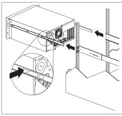
Lift the server at a slight angle, and pull it from the slide rails. Then place the server on a flat, nonconductive surface.
