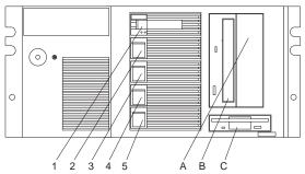
Touch the static-protective bag containing the drive to any unpainted metal surface on the server; then, remove the drive from the bag. Check the instructions that come with the drive if you need to set any switches or jumpers on the drive, or if you need to attach a tray to the drive.
