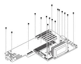
Remove the system board mounting screws to separate the system board from the back-plate.
