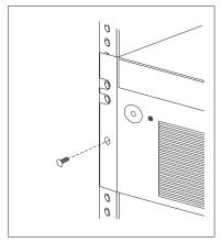
Pull the rack model out of the rack enclosure until both slide rails lock.
