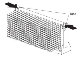
c. Lift the microprocessor out of the connector.
