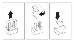
Place a jumper by aligning the holes in the bottom of the jumper with the two pins on the pin block, and then sliding the jumper onto these pins.
