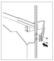
b. From the rear of the rack enclosure, insert a long screw through the holes in the cable-management arm mounting panel and cage nut; then, tighten the screws.
