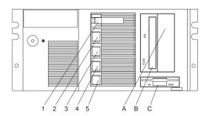
Your server comes with a CD-ROM drive installed in bay B and a diskette drive installed in bay C.
