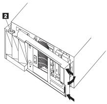
b. Press the right end of the bezel toward the server front until the bezel clicks into place.
