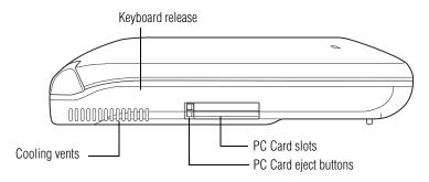
The **cooling vents** prevent the computer's central processing unit (CPU) from overheating so that it can continue to perform at its maximum speed.
