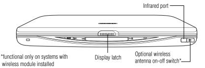
The **display latch** keeps the display panel closed and locked. To open the display panel, slide the display latch to the right and raise the panel.
