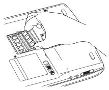
Inserting the memory module
