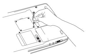
Removing the memory slot cover screws
