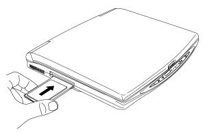
Inserting a PC Card
