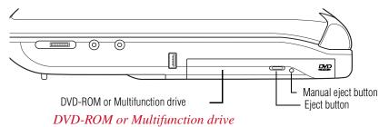
Use the eject button to release the disc tray. This button requires power to operate.
