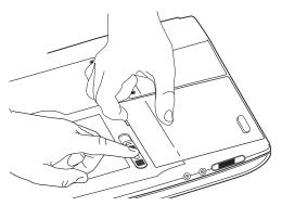
Sliding the battery release latch
