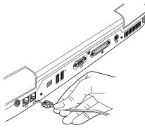
Connecting the internal modem
