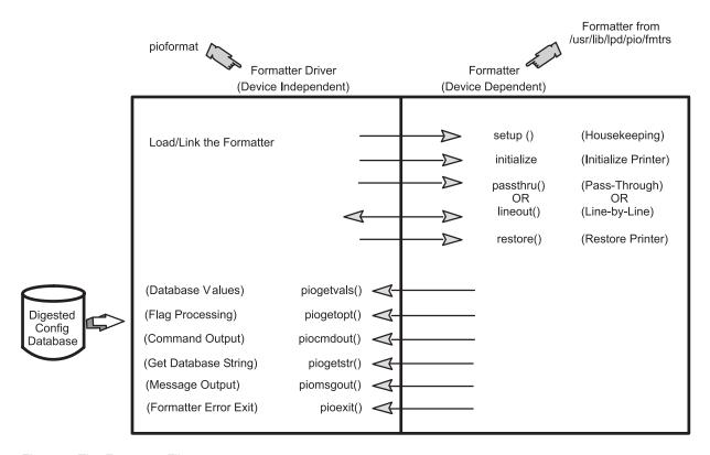
Figure 3. The Formatter Filter
