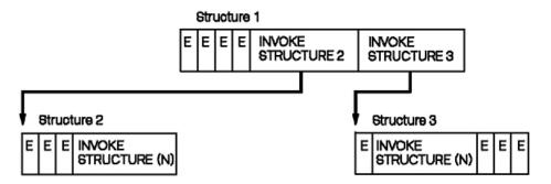
Figure 41. Results of a Delete Structure Network (GPDLNT) subroutine. This illustration shows the results of deleting a structure network.
