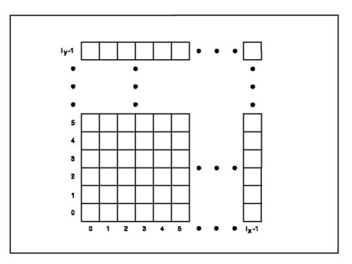
Figure 92. Accessing a frame buffer as an array of pixels. This diagram shows the configuration of a frame buffer accessed as a two-dimensional array of pixels. The array is of size  $I_X$  by  $I_y$ . The indices are from 0 to  $I_x$  - 1 and 0 to  $I_y$  - 1 respectively.
