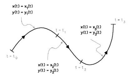
Figure 54. The piecewise polynomial representation of a curve. This illustration shows a curve made up of three spans. The first span of the curve uses  $x(t)=x_1(t)$  and  $y(t)=y_1(t)$  as its equations when t is between  $t_0$  to  $t_1$ . The second span of the curve (between  $t_1$  and  $t_2$ ) uses  $x(t)=x_2(t)$  and  $y(t)=y_2(t)$ . The third span (between  $t_2$  and  $t_3$ ) uses  $x(t)=x_3$  and  $y(t)=y_3$ . The aforementioned equations are defined in the text that follows.
