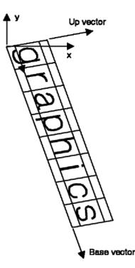
Figure 62. Rotating and shearing the text extent rectangle. This illustration depicts a series of letters in character boxes concatenated to form a parallelogram The series of letters form the word graphics. In this case, the up vector is pointing in a northeastern direction (rotated about 80 degrees from north), and the base vector points in a southeastern direction (rotated about 160 degrees from north). This causes the text to appear angled and sheared in a diagonal direction.
