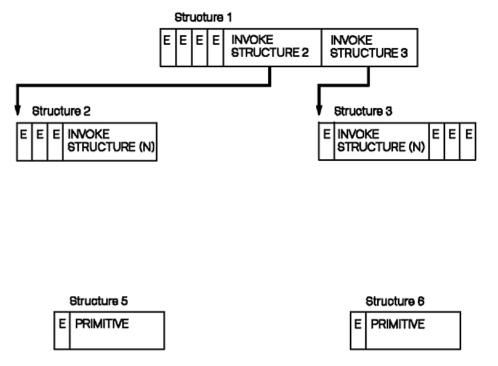
Figure 40. Results of a Delete Structure (GPDLST) subroutine. This illustration shows the results of a delete operation applied to the structure network.
