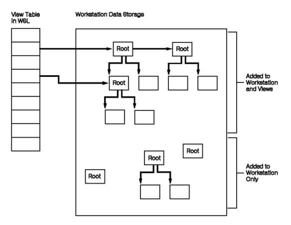
Figure 26. Workstation Capable of Storing Associated and Non-Associated Structures. This illustration shows that root structures can be associated to both a workstation and a view or to just a workstation. In this way, the workstation data is available to the workstation even if the data is not currently being displayed. Once the data is associated to the view as well as the workstation, then the graphics data will be displayed.
