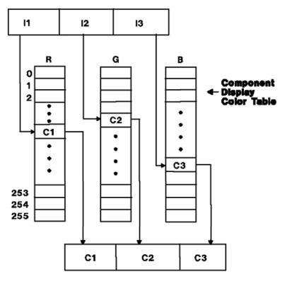
Figure 96. Component Image Board Connection. This diagram shows that the resulting color value is the color of the pixel.
