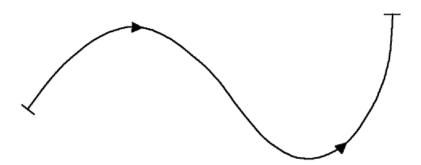
Figure 51. A 2D NURBS curve. This illustration depicts a sine curve as an example of a two-dimensional NURBS curve.
