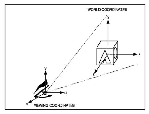
Figure 11. Relationship between the WCS and the VCS. This illustration shows an eye looking at a box. The eye is in viewing coordinates (u,v,n); the box is in world coordinates (x,y,z).
