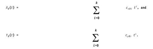
Likewise, the third span, with parameter values running from  $t_2$  to  $t_3$ , is determined by the following polynomials:
