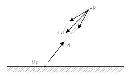
Figure 82. Spot Light Source Definition. This illustration depicts the various components of a spot light definition. The location of the spot light is denoted by  $L_p$ , and its source direction is denoted as  $L_d$ . A point on the surface which falls within the light cone is labeled as  $O_p$ . This point is illuminated; the illumination direction is depicted as an arrow pointing back to the spot light source and is denoted by  $I_d$ .
