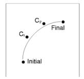
Figure 71. Third Order Bezier Curve Over Time. This illustration shows a curved line connecting two end points with two defined control points,  $C_1$  and  $C_2$ . The first end point is labeled Initial and the second end point is labeled Final. The control points are located outside the curve, and each one is evenly spaced between the two end points.
