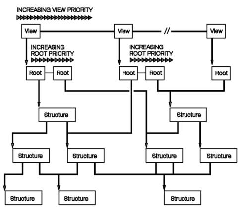
Figure 27. Structure Traversal Processing. This illustration shows how each view is traversed in the order of its assigned priority, from lowest to highest.
