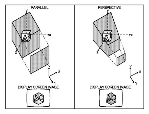
Figure 17. How Parallel and Perspective Viewing Affects Viewing Volumes and Images. Two illustrations show the difference between parallel and perspective views. The parallel illustration shows a cubic view volume and a display screen image that looks "squashed," as though the object were flattened into the screen. The perspective illustration shows a view frustum that is narrower towards the eye and wider away from the eye; the resulting display screen image has a more natural appearance.
