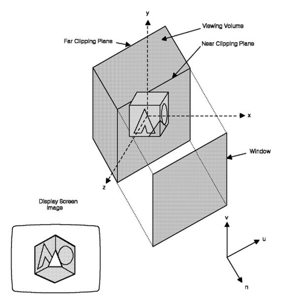
Figure 15. Modifying the Viewing Volume (Part 3 of 4). Enlarge Window and Move Near Clipping Plane. This illustration restores the initial window size, but moves the near clipping plane back until it clips the front of the object. The final display shows the object with the front edge trimmed away.
