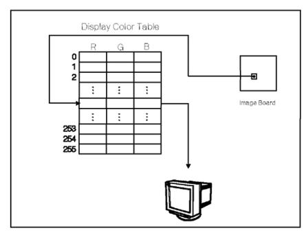
Figure 95. Vector Quantization. This diagram shows the quantization method in which color values are quantized as three-dimensional vectors.
