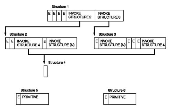
Figure 39. Results of an Empty Structure (GPEST) subroutine. This illustration shows the results of an empty operation applied to the structure network.
