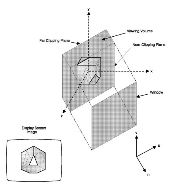
Figure 16. Modifying the Viewing Volume (Part 4 of 4). Move Far Clipping Plane. This illustration continues by moving the far clipping plane forward until it clips the back of the object. The final display shows the object with both the front and back edges trimmed away.
