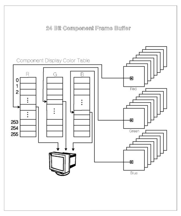
Figure 88. 24-Bit Component Frame Buffer. This diagram shows the configuration of a 24-Bit component frame buffer. There are three separate color component buffers. The component display color table contains 256 (0-255) color values for each component; that is, three tables, one for each component. This value can then be used by the display.
