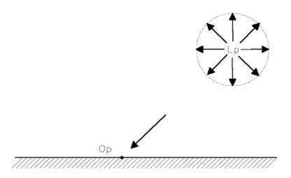
Figure 80. Positional Light Source Definition. This illustration depicts a positional light located in the upper right hand corner. The location of the light source is labeled as  $L_p$  and the light rays emitting from this source travel outward in all directions, much like the rays from the sun. A point on the surface is labeled as  $O_p$ .
