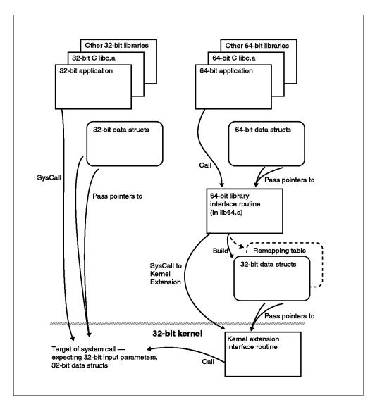
Figure 6. Interfacing 64-Bit Processes to a 32-Bit Kernel
