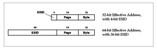
Figure 7. Effective Segment IDs in 32-Bit and 64-Bit Mode
