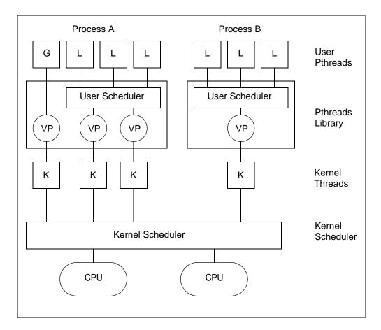
Figure 8. M:N Threads Model
