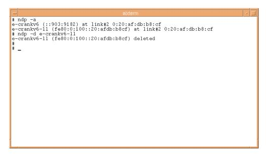
Figure 38. Example of ndp Command Usage
