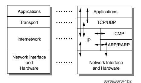
Figure 2. TCP/IP Stack
