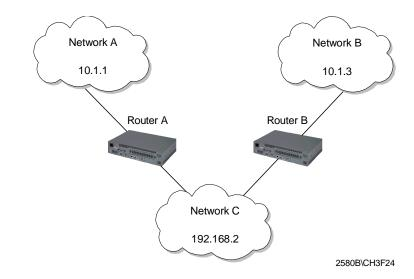
Figure 27. Routing Problems Faced with Discontinuous Networks
