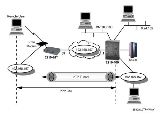
Figure 79. L2TP Tunneling Scenario with Nways Routers
