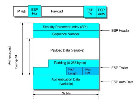
Figure 95. IPSec Encapsulating Security Payload (ESP)
