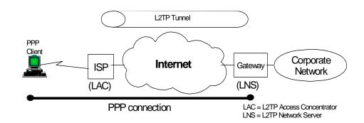
Figure 76. L2TP Compulsory Tunnel Model
