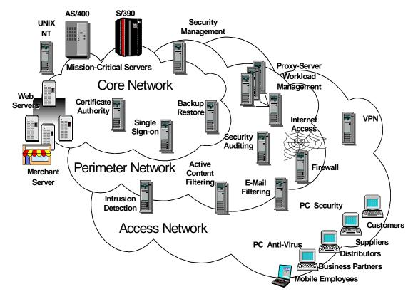
Figure 88. Network Zones and Security Components
