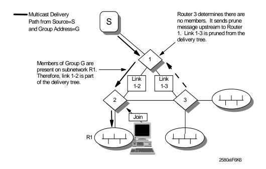
Figure 112. Reverse Path Multicasting (RPM)
