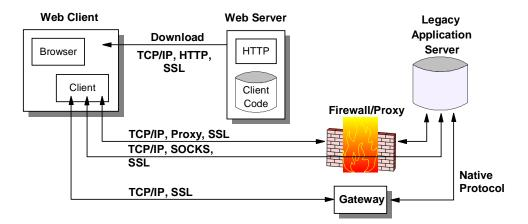
Figure 105. Web-enabled Application Using Download Client
