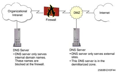
Figure 47. Implementing Internal and External Domain Name Spaces
