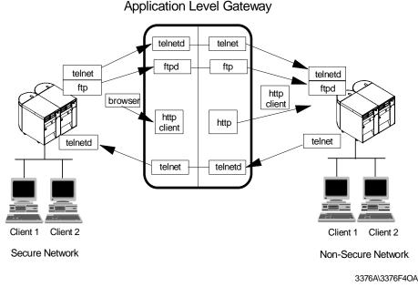
Figure 101. Application Level Gateway (Proxy Server)
