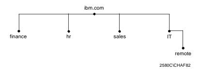
Figure 121. DNS Structure for Medium Size Network
