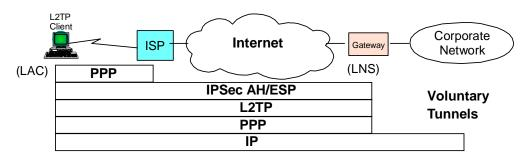
Figure 83. IPSec Protection for L2TP Voluntary Tunnel to VPN Gateway
