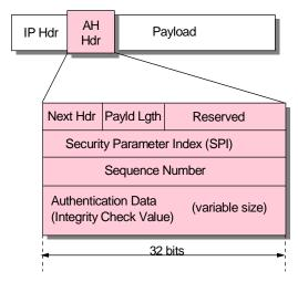
Figure 94. IPSec Authentication Header (AH)
