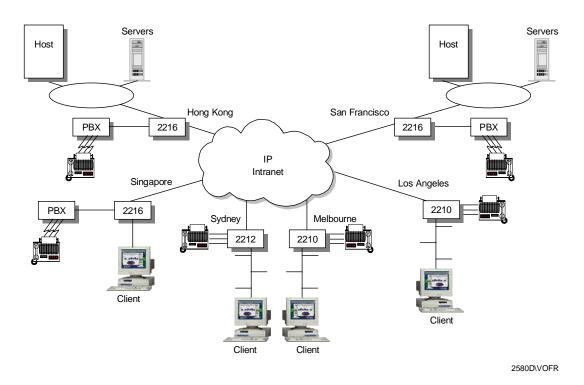
Figure 124. PBX Trunking Replacement and Toll Bypass
