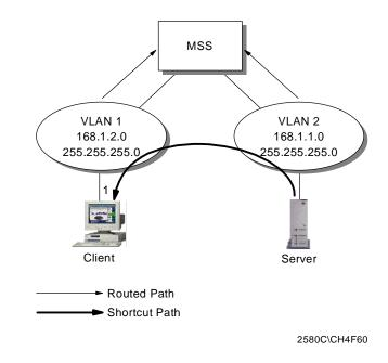
Figure 62. VLAN IP Cut-Through
