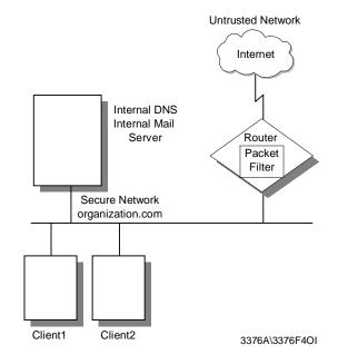
Figure 91. Packet-Filtering Router
