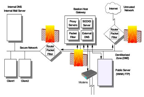
Figure 100. Screened Subnet Firewall
