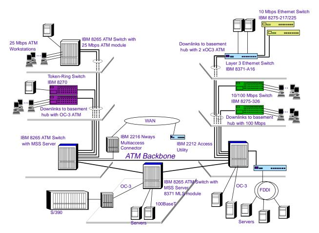
Figure 122. General Concept for a Large Network Connectivity
