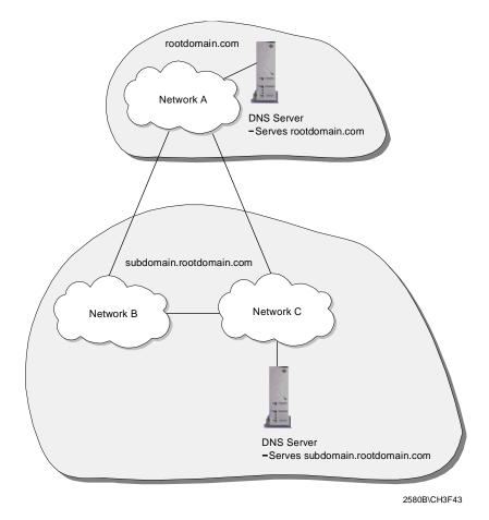
Figure 46. Internal Domain Server Allocation with Multiple DNS Servers
