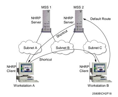
Figure 58. One-Hop Routing with NHRP
