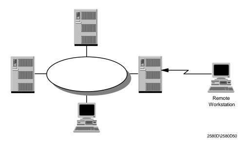
Figure 67. Remote Workstation Dial-In to LAN
