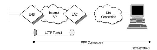
Figure 75. Layer 2 Tunnel Protocol (L2TP) Scenario
