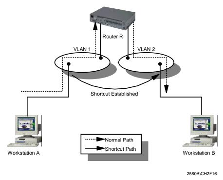
Figure 56. Router Accelerator
