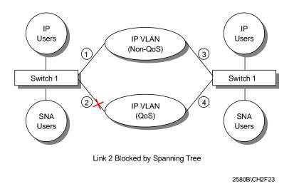
Figure 65. Network Design with Two Switches
