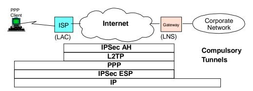
Figure 82. IPSec Protection for L2TP Compulsory Tunnel to VPN Gateway
