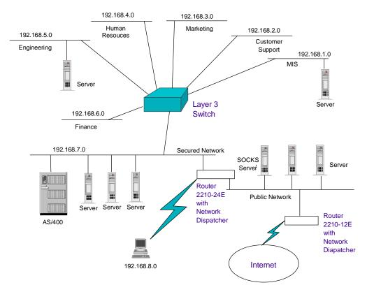
Figure 120. Logical Network Design for a Medium Size Network
