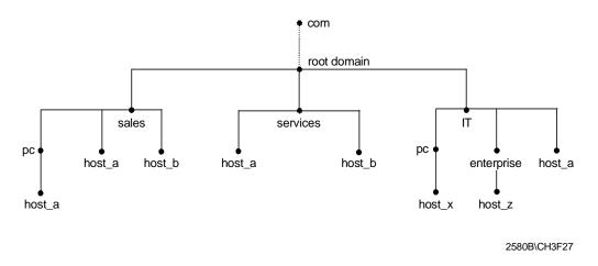
Figure 48. Badly Structured Domain Name Space and Subdomains
