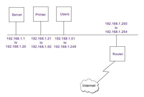
Figure 118. Logical Network Design for a Small Network
