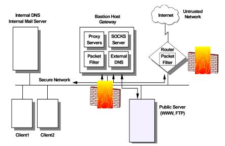
Figure 99. Screened Host Firewall
