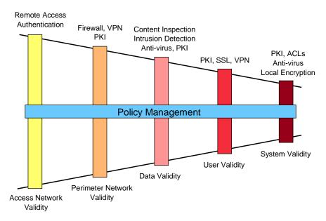
Figure 89. Placement of IP Security Technologies
