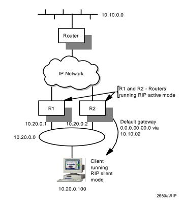
Figure 53. RIP Active and Passive Routing
