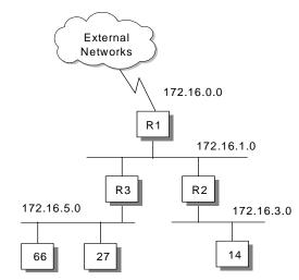
Figure 26. Subnet Configuration Example
