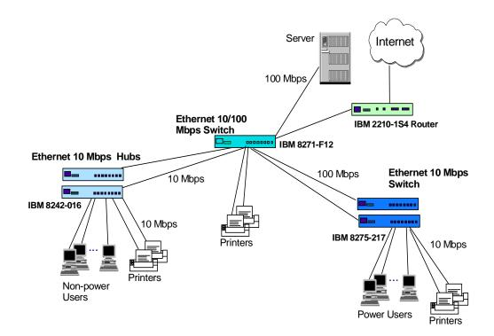
Figure 116. Physical Diagram for a Small Network - Phase 1
