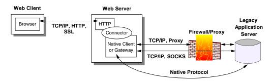
Figure 104. Web-Enabled Application Using Connectors
