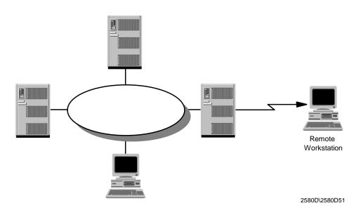
Figure 68. LAN Dial-Out to Remote Workstation
