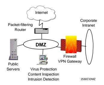
Figure 90. Demilitarized Zone (DMZ) Securing the Perimeter Network
