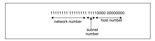
Figure 24. 4-Bit Subnet Mask for a Class B Address
