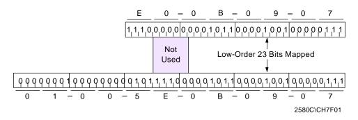
Figure 111. Mapping of Class D IP Address To MAC Address
