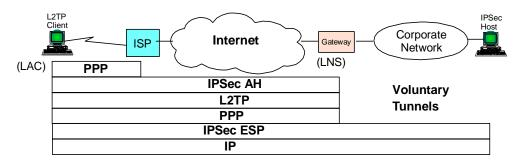
Figure 85. IPSec Protection for L2TP Voluntary Tunnel End-to-End
