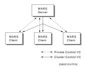
Figure 113. MARS Control Connections
