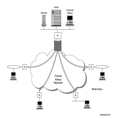
Figure 15. Star Topology in a Frame Relay Network
