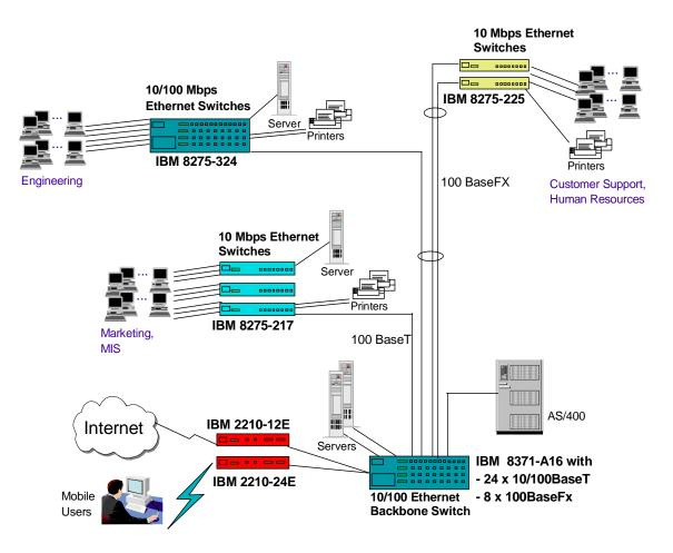
Figure 119. Connectivity Diagram for a Medium Size Network
