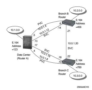
Figure 16. SVCs in a Frame Relay Network
