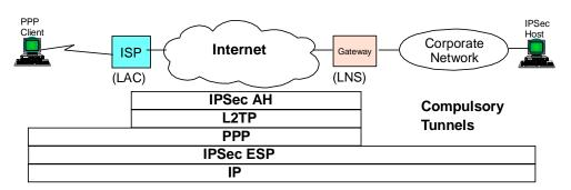
Figure 84. IPSec Protection for L2TP Compulsory Tunnel End-to-End
