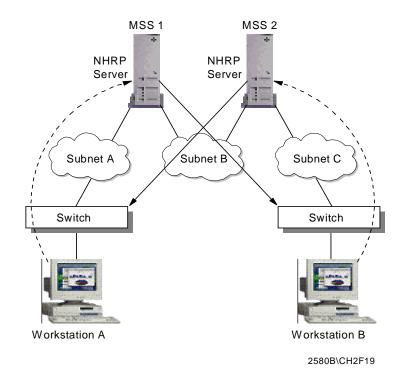
Figure 59. One-hop Routing in LANE
