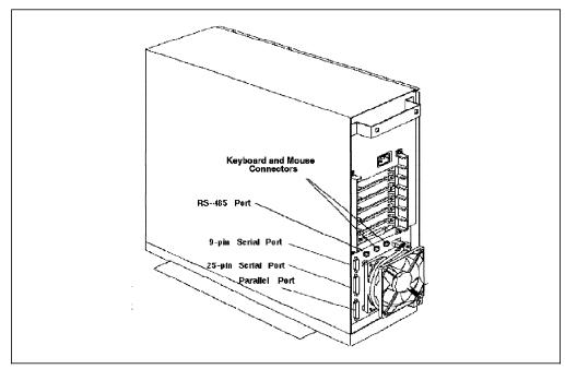
Figure 45. Rear View of the Model G40 Server
