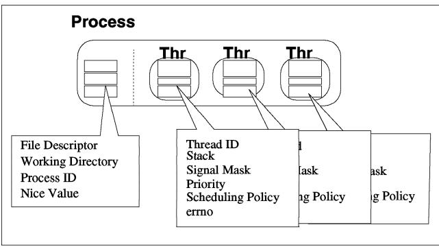
Figure 23. Threads and Processes Properties
