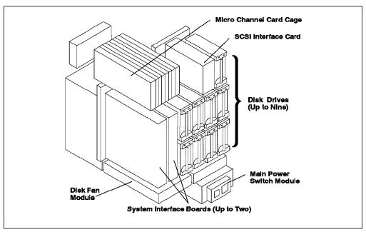
Figure 53. Rear Internal View of the J01 Expansion Cabinet
