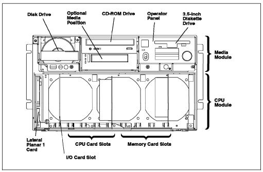
Figure 58. Front Internal View of the R40 Server
