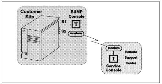
Figure 75. Console Connection
