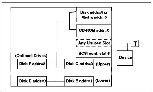
Figure 46. SCSI Device Addresses and Location for the G30 or G40 Server
