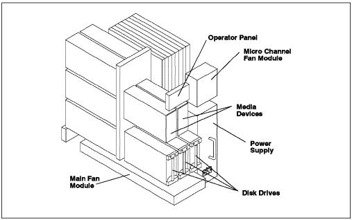
Figure 52. Front Internal View of the J01 Expansion Cabinet
