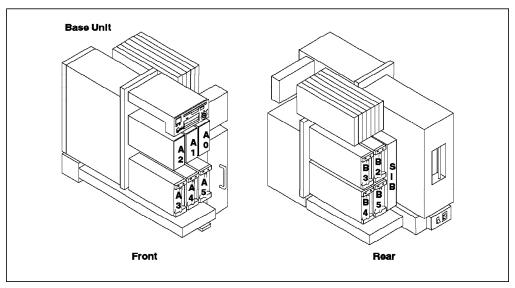
Figure 51. Front and Rear SCSI Devices Locations on the J40 Server
