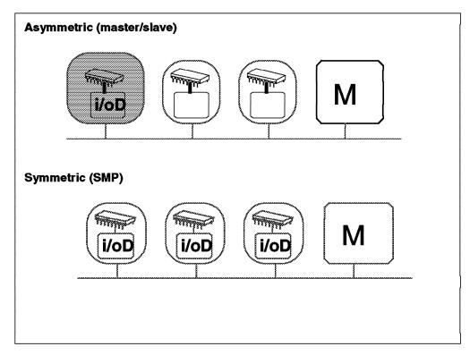
Figure 6. Symmetric versus Asymmetric Shared-Memory Multiprocessors
