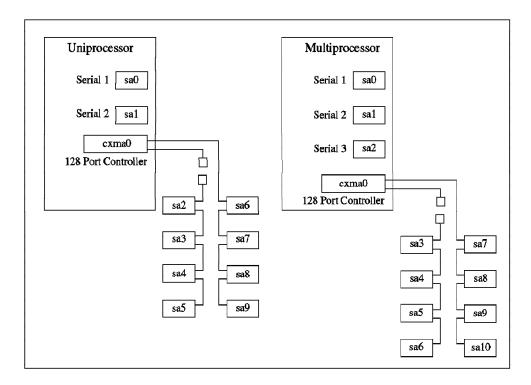
Figure 156. Asynchronous Ports Configuration
