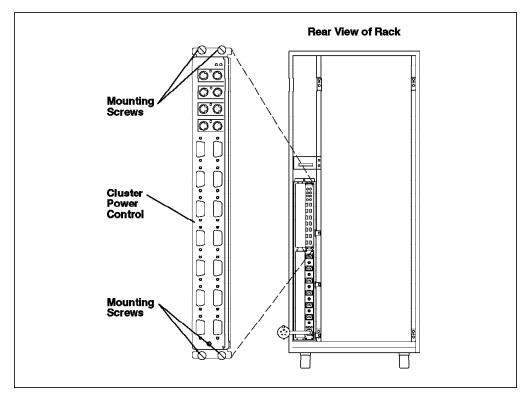
Figure 123. Rack-Mounted CPC
