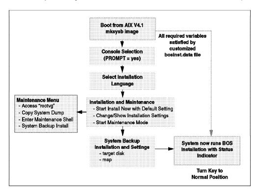
Figure 152. Installation Flow for mksysb
