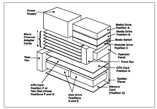
Figure 44. Internal View of the Model G30 or G40 Server
