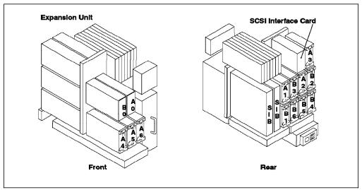
Figure 56. J01 SCSI Device Location and Addresses
