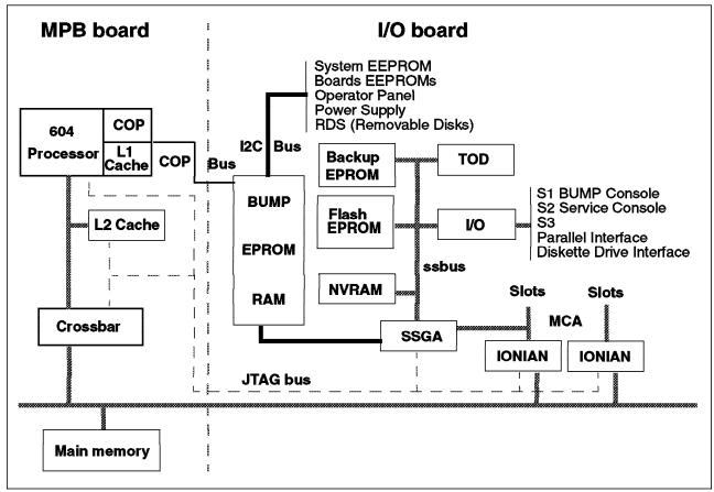
Figure 60. SystemGuard Hardware Components
