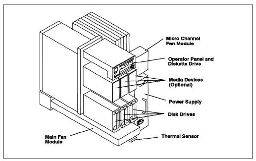
Figure 49. J40 Front Internal View
