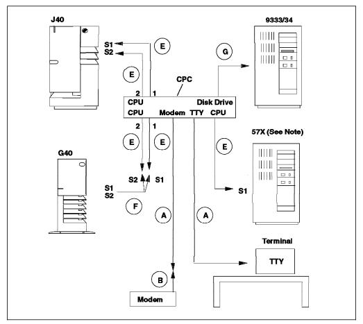
Figure 122. Multiple CPUs connected to a single CPC
