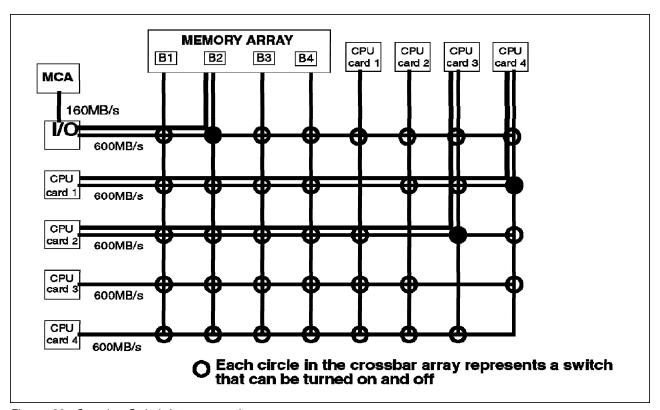
Figure 38. Crossbar Switch Interconnection
