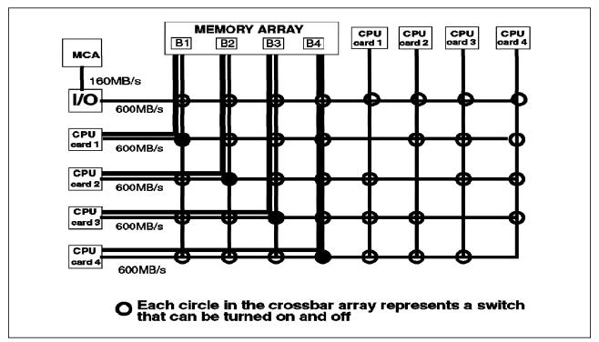
Figure 37. Crossbar Switch Interconnection
