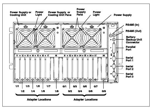
Figure 59. Rear View of the R40 Server
