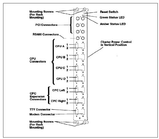
Figure 120. CPC Front Panel
