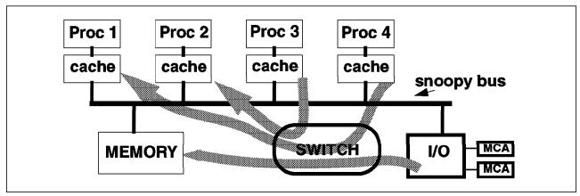
Figure 34. Using a Switch for Data Transfer
