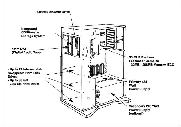
Figure 4. IBM PC Server 500 - Mechanical Design
