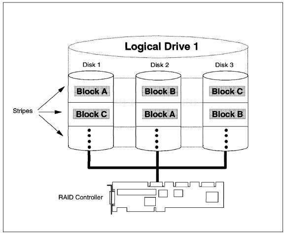
Figure 47. RAID-1, Disk Mirroring
