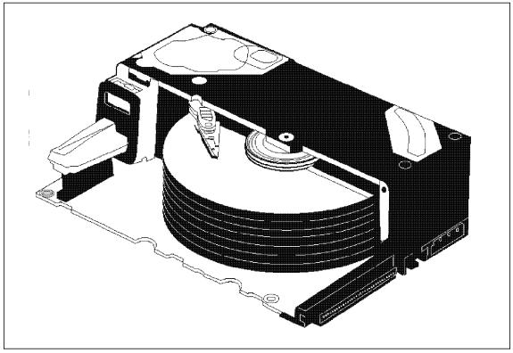
Figure 11. Ultrastar Hard Disk Drive Mechanical Design
