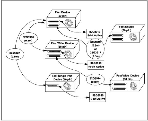
Figure 36. Option to Option Cables and Terminator Summary
