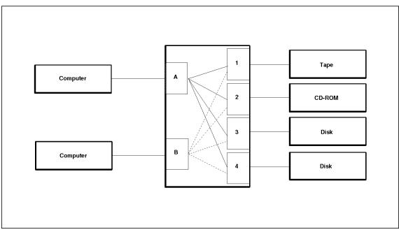
Figure 70. APPLIED Concepts (4x2 Electronic Crosspoint Switch)
