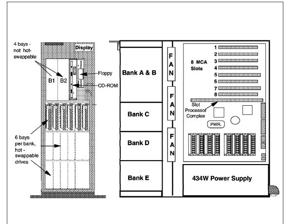
Figure 24. IBM PC Server 500 - Mechanical Design
