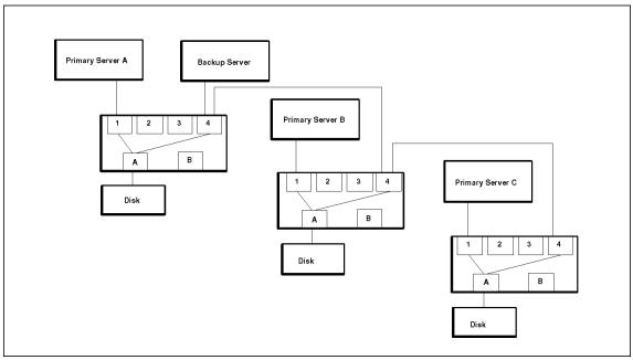
Figure 71. APPLIED Concepts (Backing up Multiple Servers)
