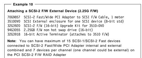
Example 10 and Figure 39 show a SCSI-2 Fast/Wide hard drive external connection.
