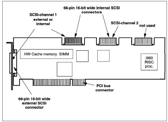
Figure 9. SCSI-2 Fast/Wide RAID PCI-Bus Adapter
