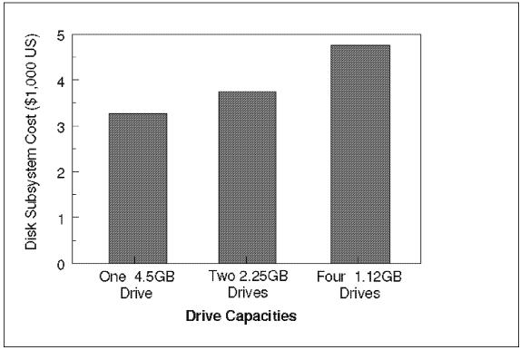
Figure 42. Disk Subsystem Cost for 4.5GB Total Capacity
