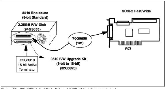
Figure 39. PCI SCSI-2 Fast/Wide External SCSI (16-bit External device)
