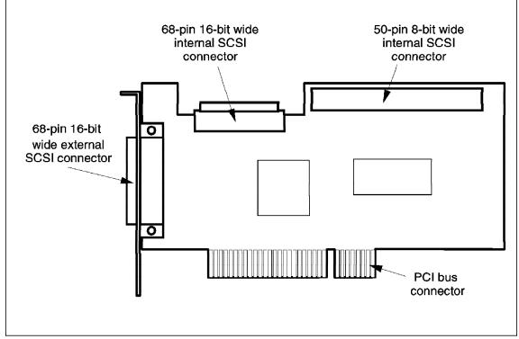
Figure 7. SCSI-2 Fast/Wide PCI Adapter
