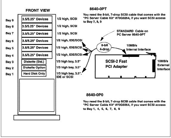
Figure 17. PC Server 300 Internal SCSI Cables
