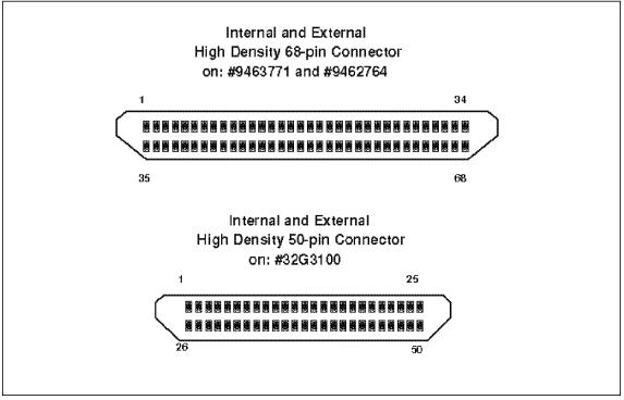
Figure 33. High Density PCI Controller SCSI Connectors
