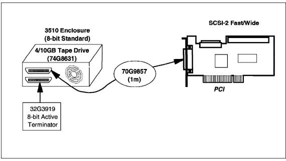
Figure 38. PCI SCSI-2 Fast/Wide External SCSI (8-bit External Device)
