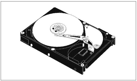
Figure 12. Deskstar Hard Disk Drive Mechanical Design
