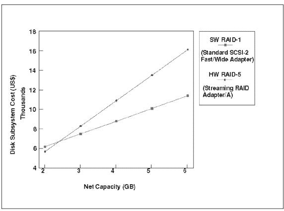
Figure 52. Cost Software RAID-1 versus Hardware RAID-5
