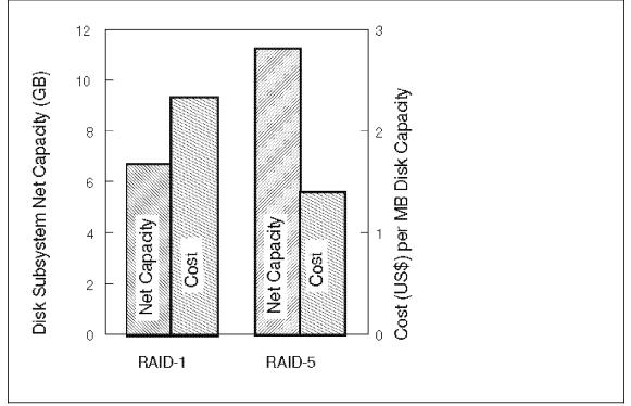
Figure 50. Disk Subsystem Cost (US Dollars/MB) for RAID-0, 1 and 5
