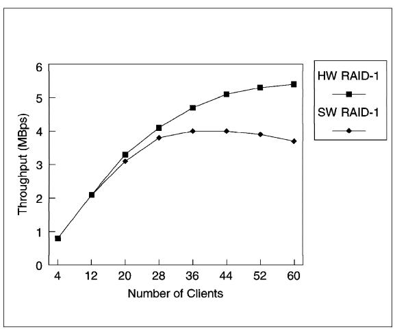
Figure 55. Software versus Hardware Mirroring
