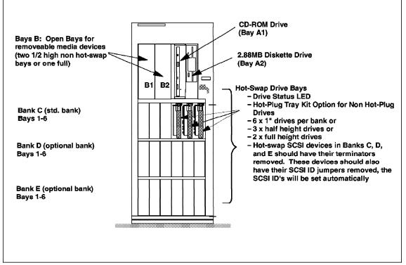
Figure 22. PC Server 500, 520, and 720 Internal Bay Structure
