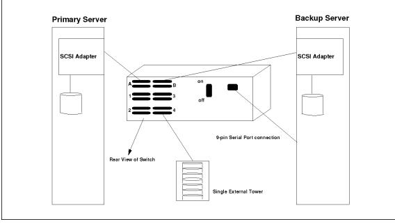
Figure 77. Sample Cabling for two CPU's
