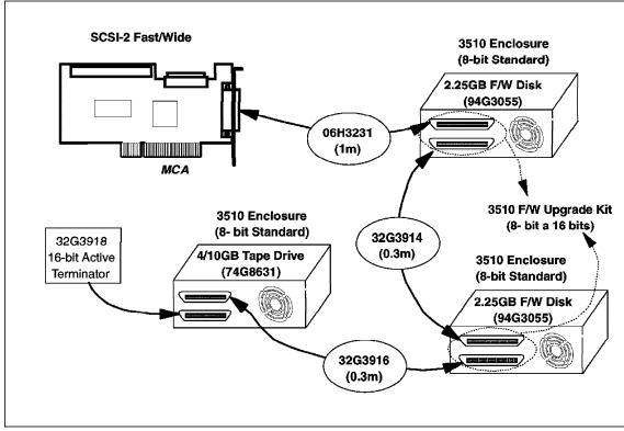
Figure 40. External 16 and 8-Bit SCSI Configuration
