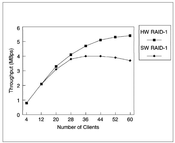
Figure 49. Software versus Hardware Mirroring
