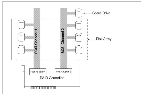
Figure 58. Disk Array Spanning Two SCSI Channels
