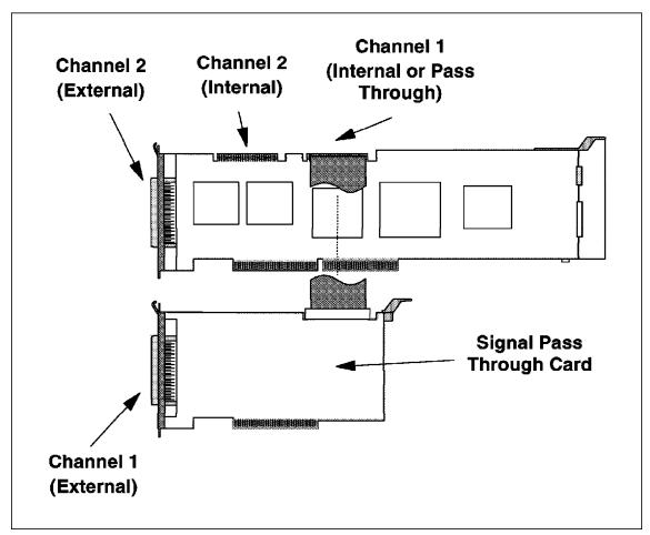
Figure 8. SCSI-2 Fast/Wide RAID Adapter Micro Channel
