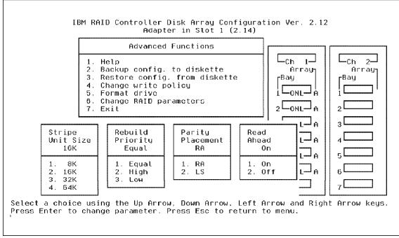
Figure 10. RAID Advanced Functions Configuration Screen
