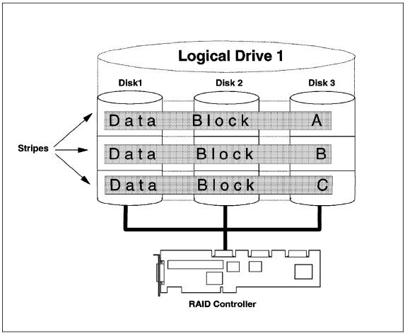
Figure 46. RAID-0, Disk Striping
