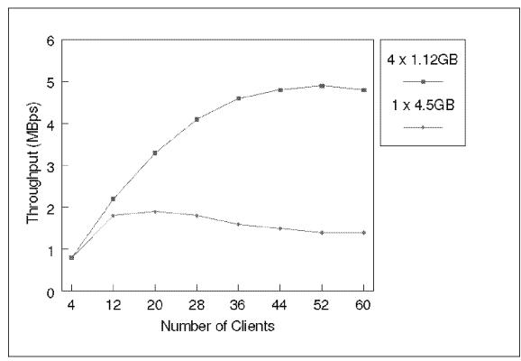
Figure 44. IBM PC Server 500 with a Single 4.5GB Drive versus Four 1.12GB Drives
