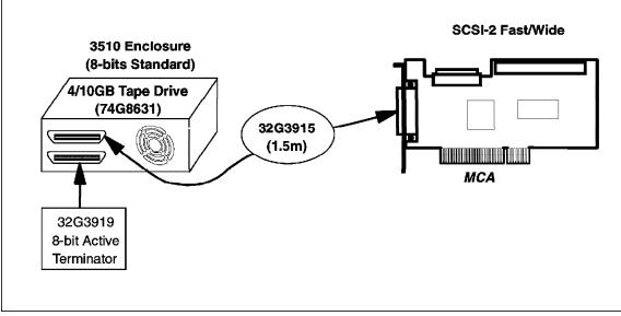
Figure 41. External 8-Bit SCSI Configuration
