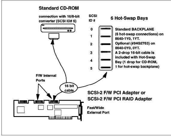
Figure 21. PC Server 320 Array or 320 with Hot Swap (SCSI-2 F/W PCI Adapter or SCSI-2 F/W PCI RAID Adapter)
