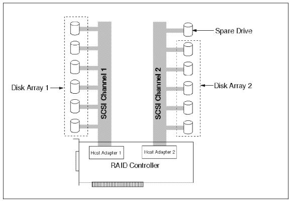
Figure 57. Disk Arrays on Separate SCSI Channels
