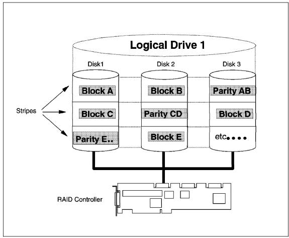
Figure 48. RAID-5, Striping Plus Parity Blocks
