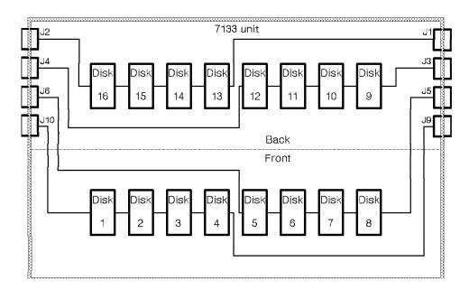
Figure 17. 7133 Disk Numbering. The order in which the disks are numbered internally.
