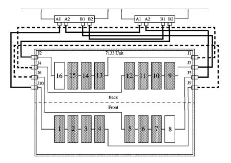
Figure 45. One Host, Two Adapters, Capacity 60 GB. This scenario illustrates a design for high availability of the disk subsystem with one host, two adapters and 60 GB of storage.
