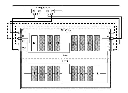
Figure 40. One Host, One Adapter, Capacity 60 GB. This scenario illustrates a design for high availability of the disk subsystem with one host, one adapter and 60 GB of storage.
