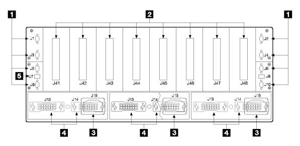
Figure 10. IBM 7133 Back Connectors. The location of the back connectors on the 7133 model 010.
