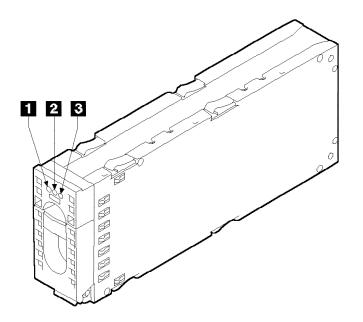
Figure 14. SSA Disk Drive Module. The physical layout of an SSA disk drive module.
