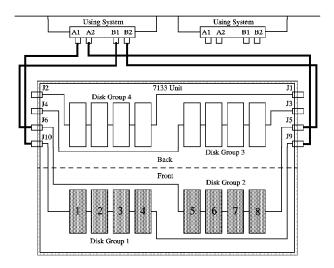
Figure 28. Eight Disk Configuration. Two loops, balanced.
