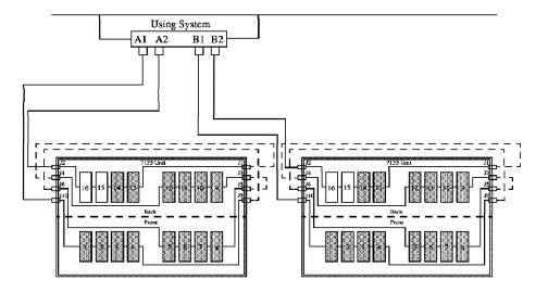
Figure 41. One Host, One Adapter, Capacity 120 GB. This scenario illustrates a design for high availability of the disk subsystem with one host, one adapter and 120 GB of storage.
