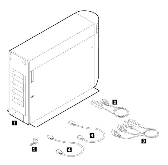
Figure 22. The 7133 Model 500. The parts required to install the 7133 model 500.
