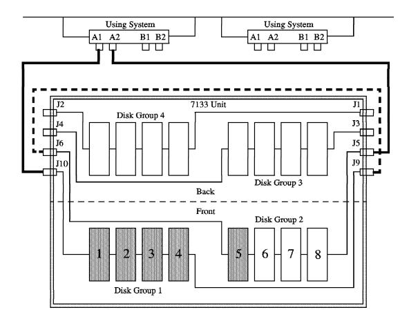
Figure 33. Sequential Access, Capacity 20 GB. This scenario illustrates a design for access to 20GB.
