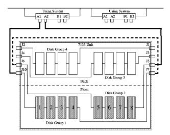
Figure 27. 8 Disk Configuration. All eight disks in one loop.
