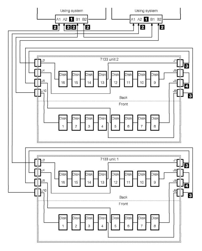
Figure 18. Dual 7133 Configuration. An example of the connections for two 7133 subsystems.
