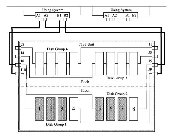
Figure 39. One Host, One Adapter, Capacity 20 GB. This scenario illustrates a design for high availability of the disk subsystem with one host, one adapter and 20 GB of storage.
