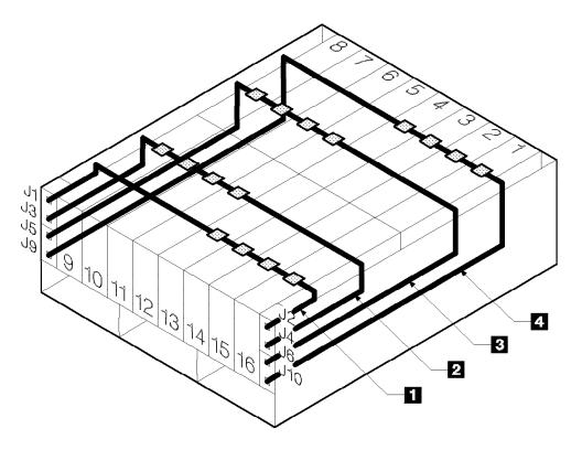
Figure 16. IBM 7133 Hardware Schematic. The layout of the disks and connectors inside the 7133.
