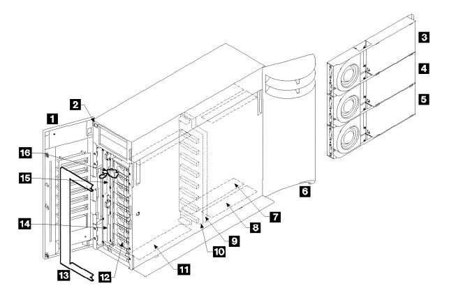
Figure 12. IBM 7133 Component Location. The location of the internal components of the 7133 model 500.
