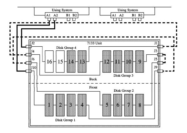
Figure 34. Sequential Access, Capacity 60 GB. This scenario illustrates a design for access to 60 GB.
