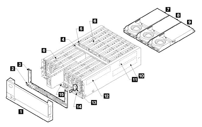
Figure 9. IBM 7133 Component Location. The location of the internal components of the 7133 model 010.
