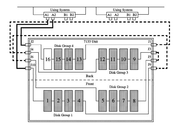
Figure 36. Random Access, Capacity 20 GB. This scenario illustrates a design for access to 20 GB.
