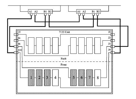
Figure 43. One Host, Two Adapters, Capacity 20 GB. This scenario illustrates a design for high availability of the disk subsystem with one host, two adapters and 20 GB of storage.
