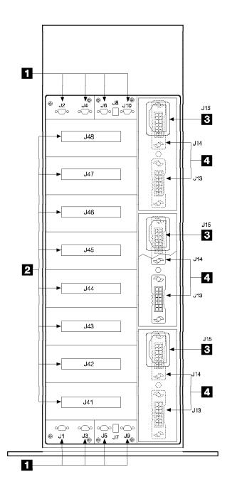
Figure 13. IBM 7133 Back Connectors. The location of the back connectors on the 7133 model 500.
