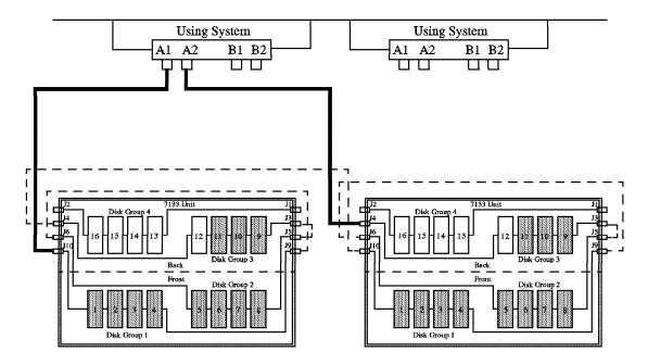
Figure 37. Random Access, Capacity 60 GB. This scenario illustrates a design for access to 60 GB.
