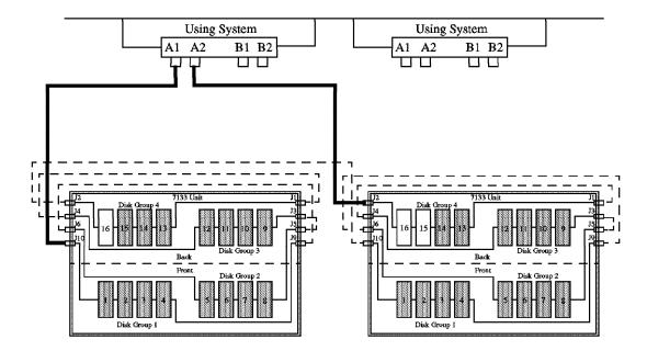
Figure 38. Random Access, Capacity 120 GB. This scenario illustrates a design for access to 120 GB.
