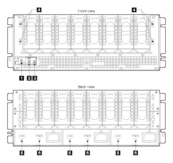
Figure 8. IBM 7133 Lights and Power. The location of the indicator lights and power switch.
