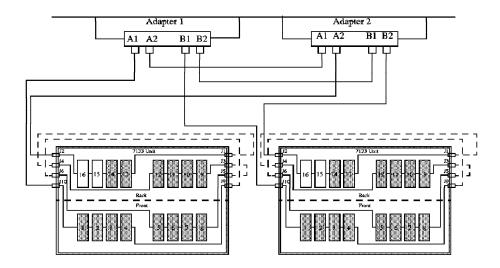
Figure 47. One Host, Two Adapters, Capacity 120 GB. This scenario illustrates a design for high availability of the disk subsystem with one host, two adapters and 120 GB of storage.
