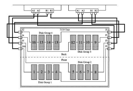
Figure 46. One Host, Two Adapters, Capacity 60 GB. This scenario illustrates a design for high availability of the disk subsystem with one host, two adapters and 60 GB of storage.
