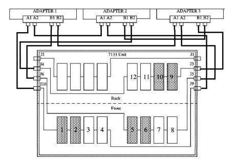
Figure 44. One Host, Three Adapters, Capacity 20 GB. This scenario illustrates a design for high availability of the disk subsystem with one host, three adapters and 20 GB of storage.
