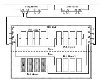
Figure 24. A Basic 7133 Configuration. An example of a simple four disk 7133 configuration
