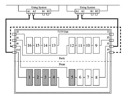
Figure 42. One Host, Two Adapters, Capacity 20 GB. This scenario illustrates a design for high availability of the disk subsystem with one host, two adapters and 20 GB of storage.
