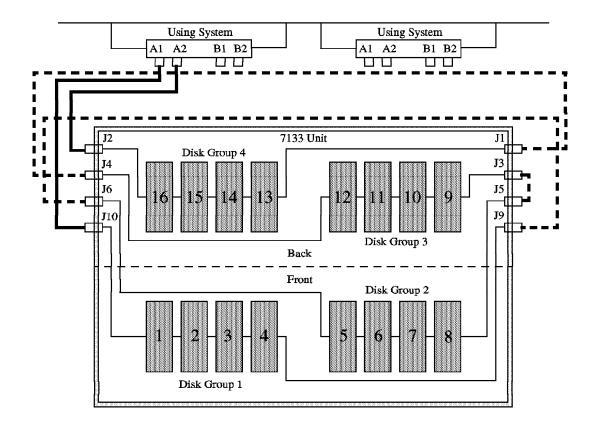
Figure 32. Multiple Adapters Example. An example configuration involving multiple adapters.
