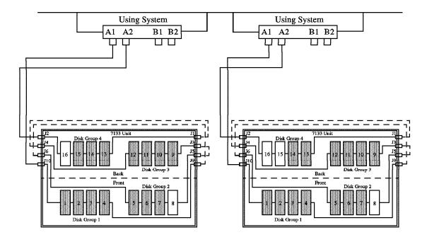
Figure 35. Sequential Access, Capacity 120 GB. This scenario illustrates a design for access to 120 GB.
