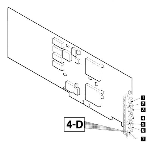
Figure 15. SSA Four-Port Adapter. The physical layout of the SSA four-port adapter.
