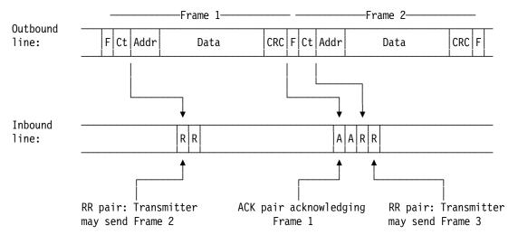
Figure 5. Flow Control. The operation for half duplex is shown. For full duplex, the ACK and RR pairs would be interspersed within the frames on the inbound signal.
