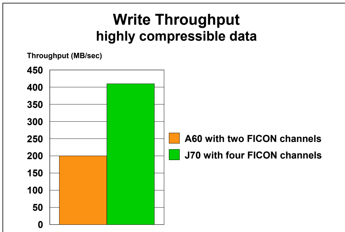
Figure 2-22 J70 and A60 write throughput comparison
