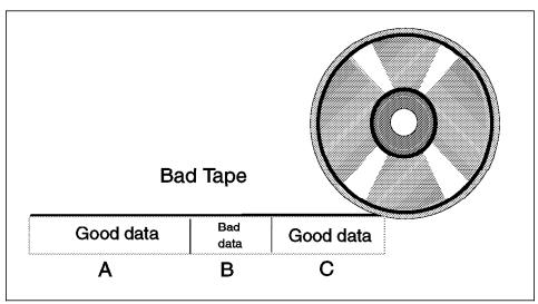
Figure 14. Damaged Storage Pool Volume Recovery
