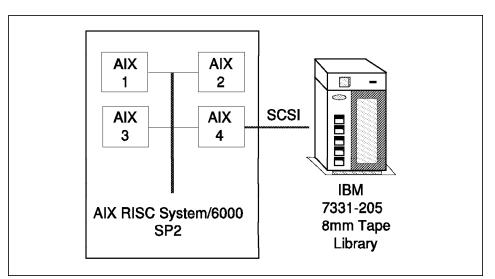
Figure 3. Single SCSI Tape Device Connected to Several AIX Systems
