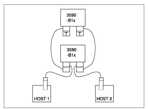
Figure 12. Sharing Two Twin-Tailed Drives between Two Hosts
