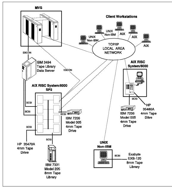
Figure 5. Mixed MVS and AIX Tape Environment
