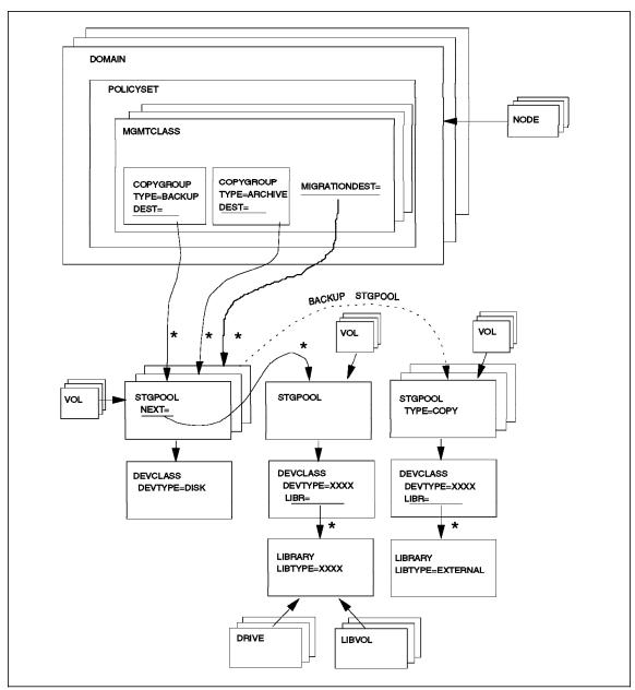
Figure 13. ADSM Server Structure
