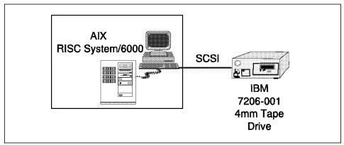
Figure 1. Single AIX System with SCSI Tape Device
