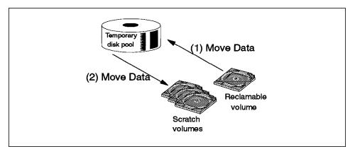
Figure 15. Single Drive Reclamation Process
