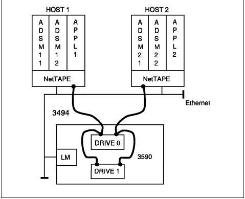
ADSM servers running on two hosts and other AIX applications. The hosts are accessing multitail drives, in this example 3590s in a 3494 ATLDS.
