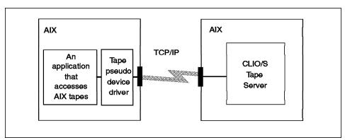
Figure 32. Accessing AIX Tapes from AIX with the Tape Pseudo Device Driver
