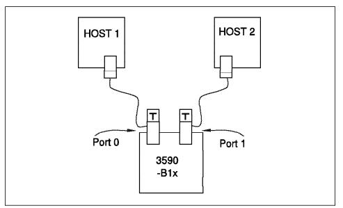
Figure 11. Two Hosts Accessing One Twin-Tailed Tape Drive
