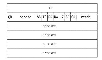
The DDNS header format has added the AD and CD bits to the original DNS header format. The AD (authentic data) bit is used by a DDNS server to indicate that it has verified the data in a message. The CD (checking disabled) bit is used by a DDNS client to indicate that it will accept data from old DNS servers (non-verified data) as well as from secure DDNS servers.
