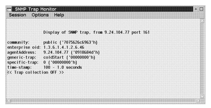
Figure 270. SNMPTRAP Showing a Trap
