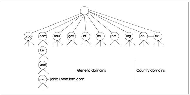
The DNS name space is hierarchical, as shown in Figure 8 on page 15.
