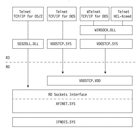
Figure 180. DOS/Windows Access Protocol Stack
