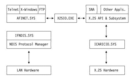
Figure 211. Communications Manager X.25 Subsystem Used by TCP/IP for OS/2
