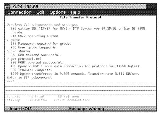
Figure 171. Transferring a File from OS/400 to OS/2 Using FTP
