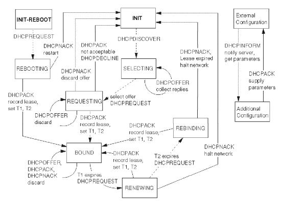
Figure 21. DHCP Client State Transition Diagram
