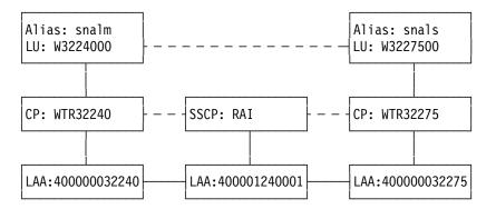
Figure 257. OS/2 to OS/2 Workstation via VTAM SNALINK Configuration
