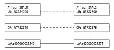
Figure 234. OS/2 to OS/2 Workstation SNALINK Configuration
