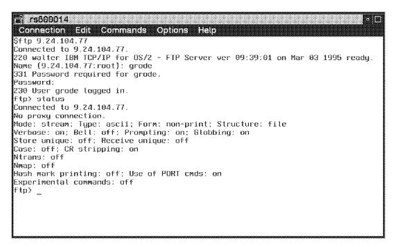
Figure 165. FTP Status on AIX Command Shell
