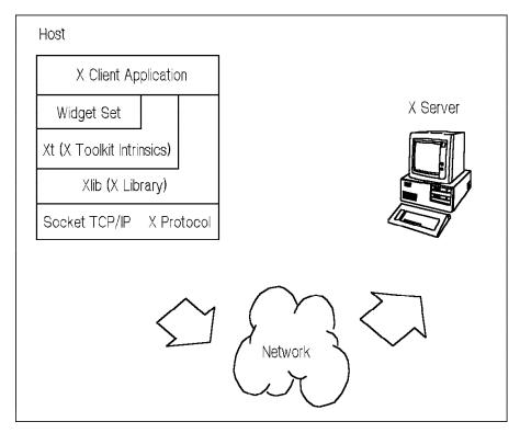
Figure 201. X Window Application Layers
