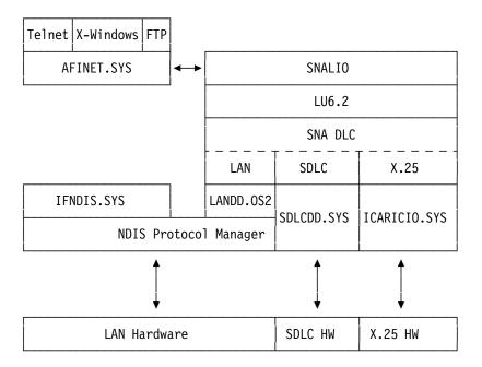
Figure 233. TCP/IP over SNALINK Protocol Stack
