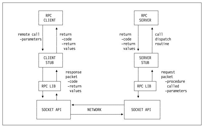
Figure 266. The RPC Mechanism
