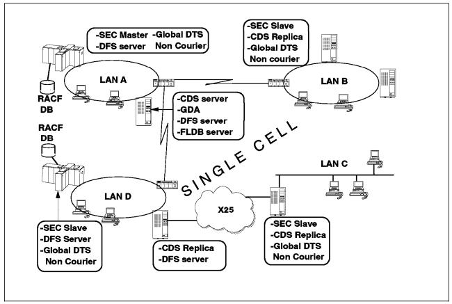
Figure 10. Scenario 2A - DCE Servers Layout. Single Cell Design - WAN Structure.
