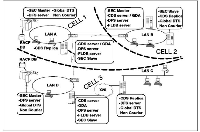
Figure 11. Scenario 2B - DCE Servers Layout. Multiple Cell Design - WAN Structure.
