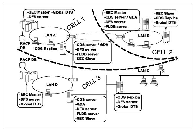
Figure 8. Scenario 1B DCE Servers Layout. Multiple Cells Design over a LAN Structure.
