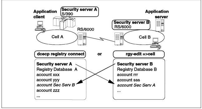
Figure 21. Security Definition in Multiple Cells Configuration. Cross Cell Trust Relationships Creation from OS/390 or from AIX.
