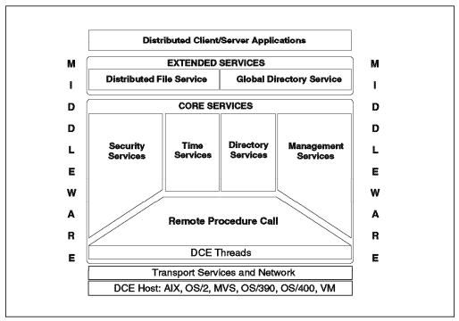
Figure 2. DCE Architecture
