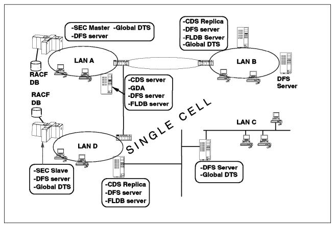
Figure 7. Scenario 1A - DCE Servers Layout. Single Cell Design over a LAN Structure.
