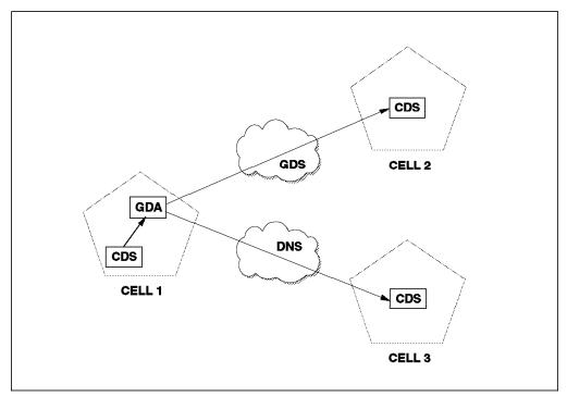
Figure 13. Interaction of CDS and GDA. The GDA helps CDS to resolve names in other cells that are registered in GDS or DNS.
