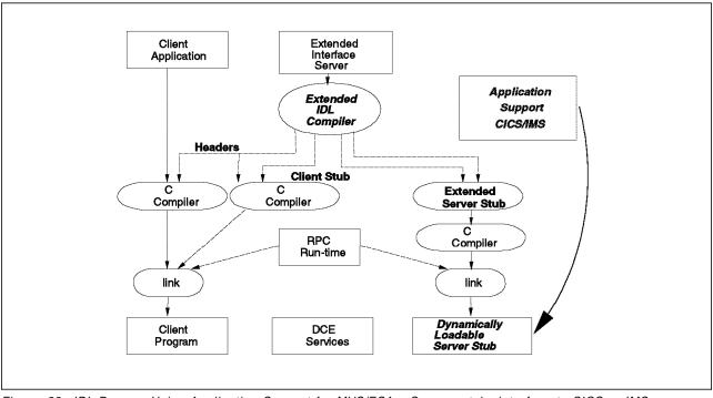
Figure 22. IDL Process Using Application Support for MVS/ESA. Servers stubs interface to CICS or IMS transactions.
