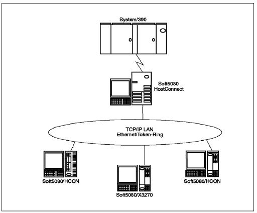
Figure 53. Hardware Topology Using HostConnect
