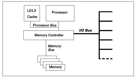
Figure 4. Simplified System Architecture: Focus on Buses
