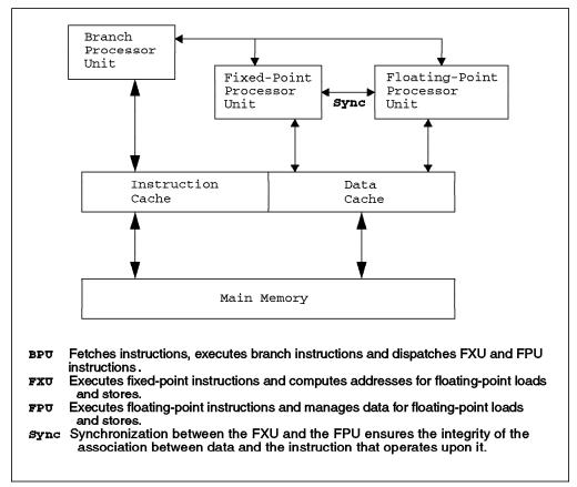
Figure 2. Pipelined Architecture
