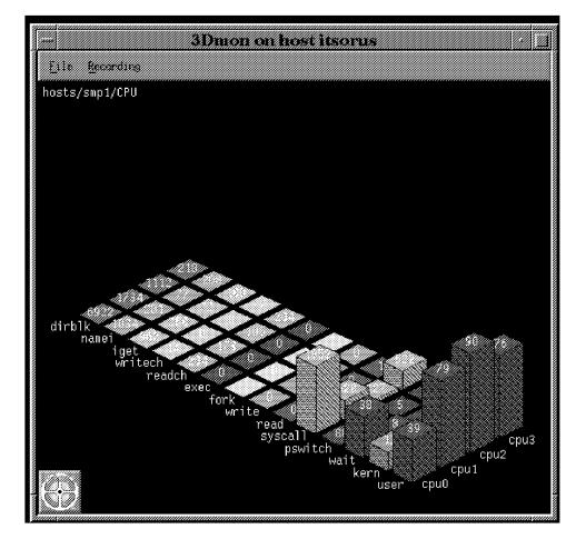
Figure 108. 3dmon Output on a 4-Way SMP
