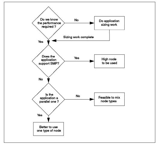
Figure 54. Performance-Based Node Selection Diagram
