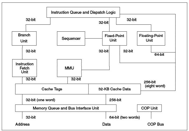
Figure 15. The PowerPC 601 Microprocessor
