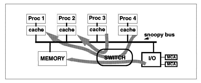
Figure 43. Using a Switch for Data Transfer
