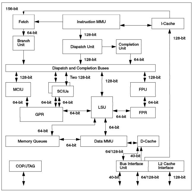
Figure 18. The PowerPC 620 Microprocessor
