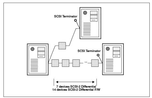
Figure 31. SCSI-2 Differential Sample
