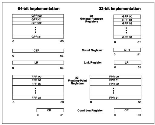
Figure 10. Comparison of 32-bit and 64-bit PowerPC Processors
