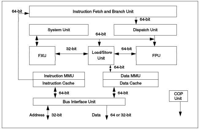
Figure 16. The PowerPC 603 Microprocessor
