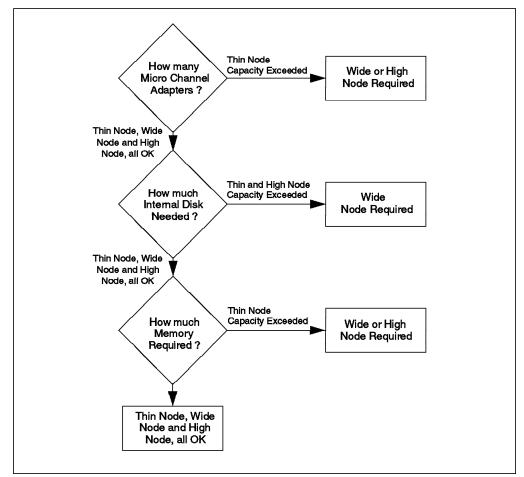
Figure 53. Capacity-Based Node Selection Diagram
