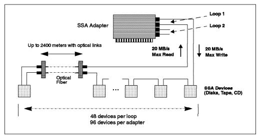
Figure 32. SSA Adapter for the RS/6000
