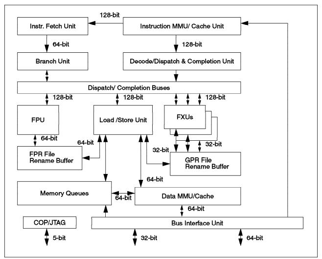
Figure 17. The PowerPC 604 and 604e Microprocessor
