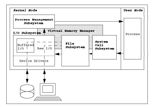
Figure 8. AIX Version 4 Kernel Subsystems
