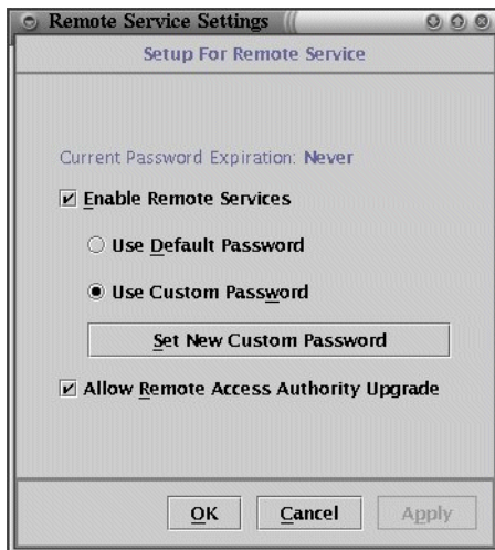
Figure 3-6 ESS Master Console: Enabling remote services
