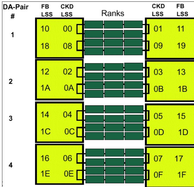
Figure 15-3 Relationship between LSSs DAs and SSA loops
