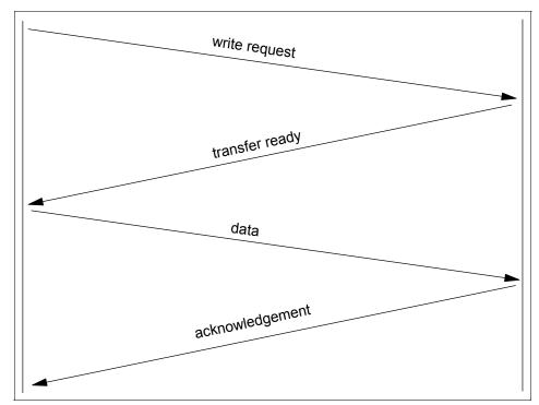
Figure 5-4 A standard write request
