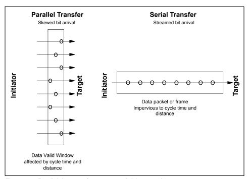
Figure 3-4 Parallel data transfers versus serial data transfers
