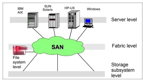
Figure 7-6 Levels that storage virtualization can be applied at
