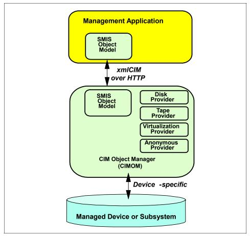
Figure 7-3 CIMOM component structure
