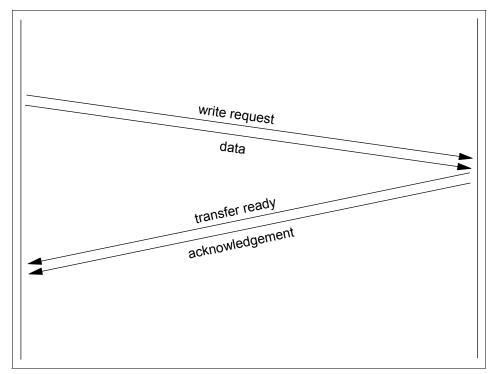
Figure 5-5 Write acceleration or Fast Write request
