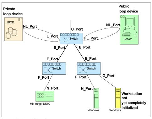
Figure 4-5 Fibre Channel port types
