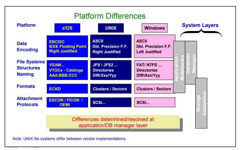
Figure 2-7 Hardware and operating systems differences
