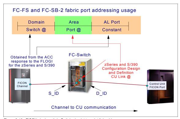
Figure 3-12 FICON single switch: Switched point-to-point link address
