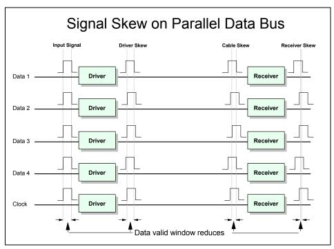
Figure 3-1 SCSI Propagation delay results in skew
