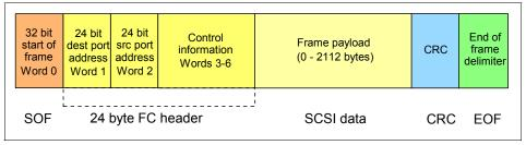
Figure 3-8 Fibre Channel frame structure
