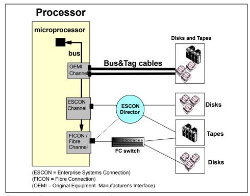
Figure 2-3 Processor-to-storage interface connections
