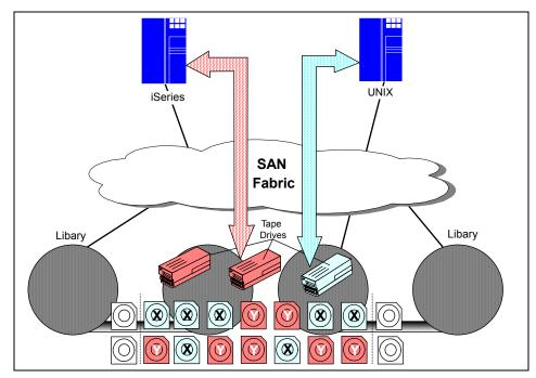
Figure 10-2 Tape pooling
