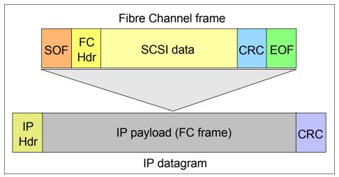
Figure 5-1 FCIP encapsulates the Fibre Channel frame into IP packets
