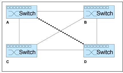
Figure 6-9 Four-switch fabric
