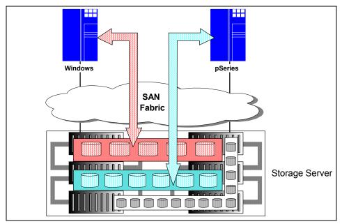
Figure 10-1 Disk pooling
