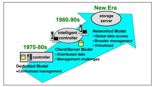
Figure 2-1 The evolution of storage architecture
