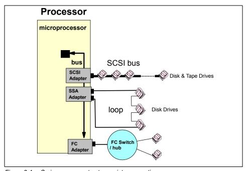
Figure 2-4 pSeries processor-to-storage interconnections
