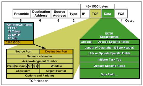
Figure 5-3 iSCSI packet format
