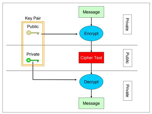
Figure 8-2 Securing a message using asymmetric cryptography
