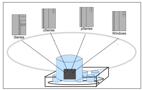
Figure 10-6 Heterogeneous data sharing
