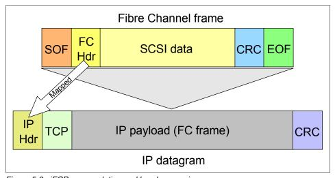
Figure 5-2 iFCP encapsulation and header mapping
