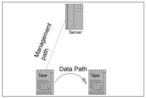
Figure 10-11 Server-free data movement for tape reclamation
