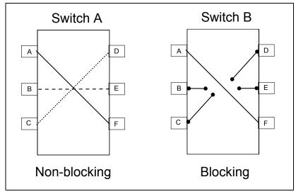
Figure 6-10 Non-blocking and blocking switching
