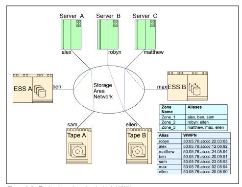
Figure 8-5 Zoning based on the device's WWN
