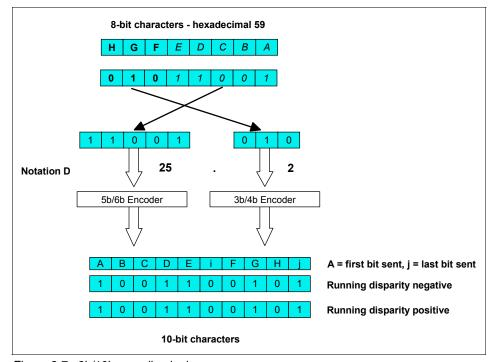
Figure 3-7 8b/10b encoding logic
