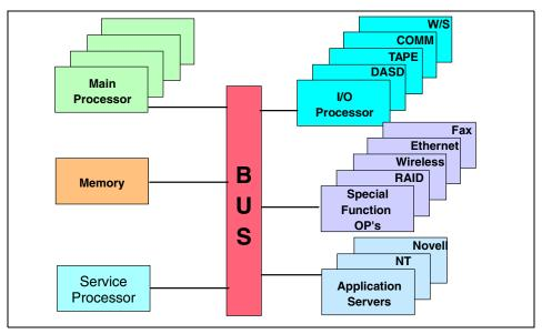
Figure 2-5 iSeries hardware design
