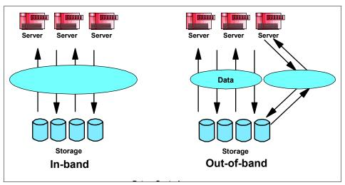
Figure 7-1 In-band and out-of-band models
