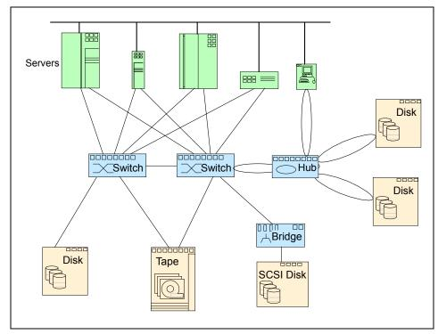
Figure 4-4 Sample switched fabric configuration
