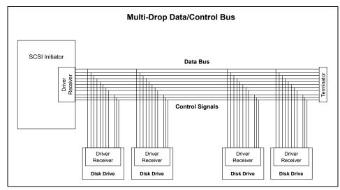
Figure 3-3 Multi-drop bus structure
