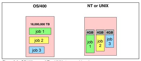
Figure 2-6 OS/400 versus NT or UNIX storage addressing
