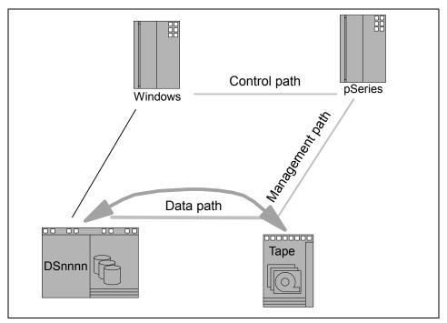
Figure 10-10 Server-free data movement for backup and recovery
