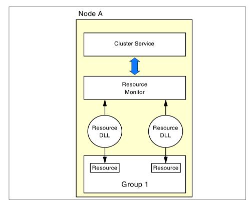
Figure 6. Communication between the Cluster Service and the resources
