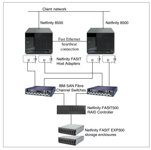
Figure 73. Two-node MSCS cluster with a fully redundant Fibre Channel disk subsystem
