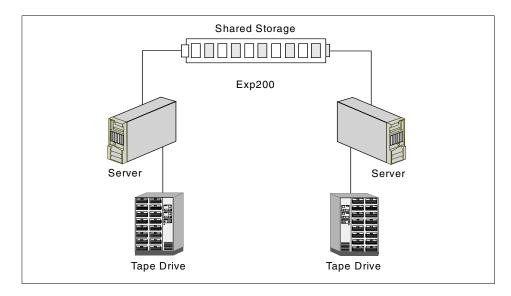
Figure 78. Tape drive configuration in a cluster
