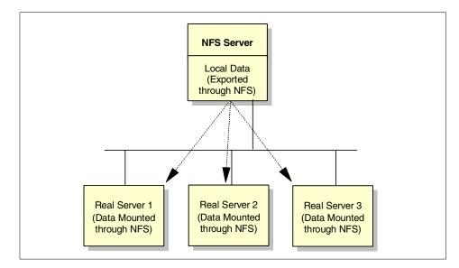
Figure 29. Using NFS for central data storing
