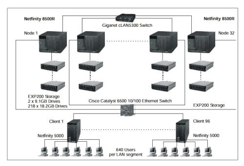
32 Netfinity servers running Windows 2000 were used for the test as shown in Figure 46, producing the TPC-C results.
