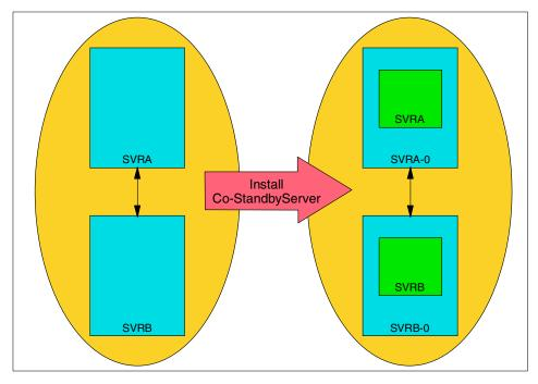
Figure 17. Effect of Co-StandbyServer on network names
