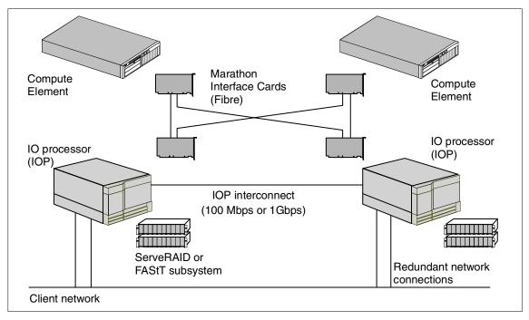
Figure 18. Marathon Endurance array — example configuration
