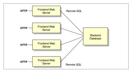
Figure 32. A cluster of front-end servers in conjunction with a fault-tolerant back-end database
