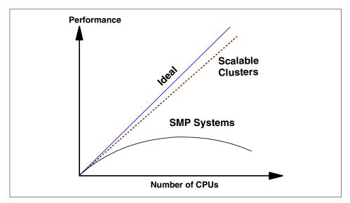
Figure 3. Scalable clusters versus SMP machines
