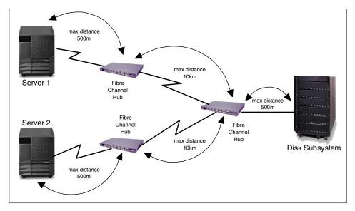
Figure 83. Maximum distance using Fibre Channel
