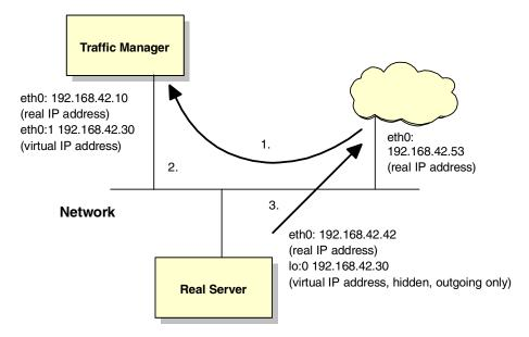
Figure 24. Direct routing of returned packets
