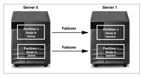
Figure 49. DB2 UDB EEE and MSCS: hot standby failover configuration
