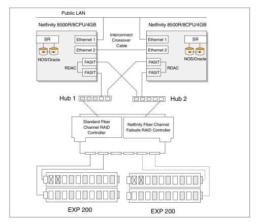
Figure 42. OPS two-node configuration
