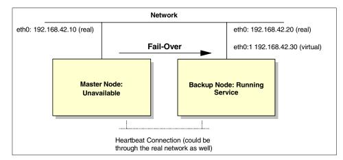
Figure 21. Failover service showing actual fail-over operation
