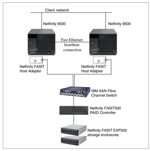
Figure 72. Two-node MSCS cluster using Fibre Channel disk subsystems
