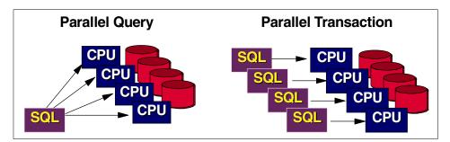
Figure 48. DB2 parallel query versus parallel transaction
