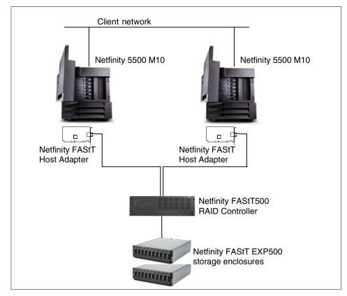
Figure 71. IBM FAStT disk subsystem for two-node clusters
