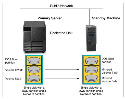
Figure 34. Novell StandbyServer configuration
