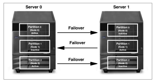
Figure 50. DB2 UDB EEE and MSCS: mutual takeover failover configuration
