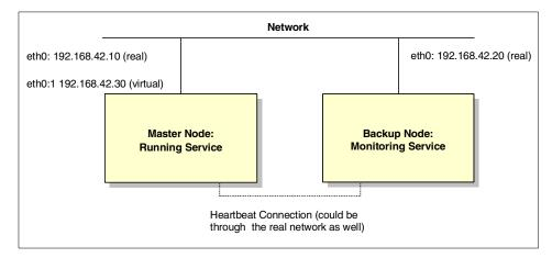
Figure 20. Failover service in normal operation
