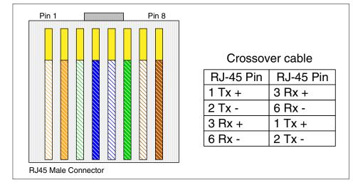
Figure 85. Ethernet 10/100 Base-T crossover cable wiring
