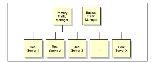
Figure 23. Simple Linux Virtual Server setup
