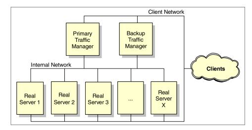
Figure 25. More sophisticated setup using an internal cluster network
