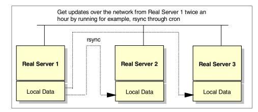
Figure 28. Using rsync for local server data synchronization
