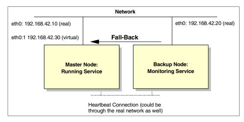
Figure 22. Failover service, resumption of normal operation
