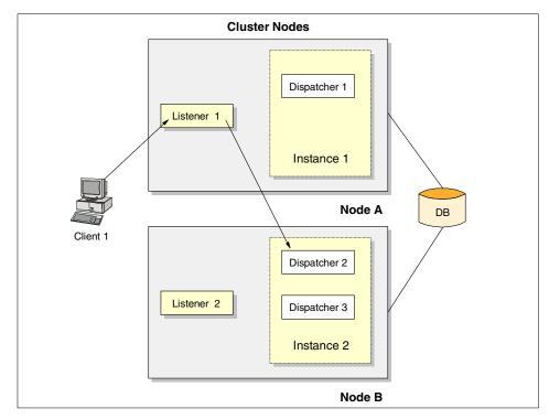
Figure 43. Connection load balancing scheme
