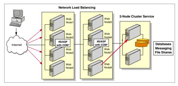
Figure 11. Example of both technologies being deployed
