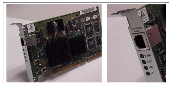
Figure 76. IBM Netfinity Gigabit Ethernet Adapter
