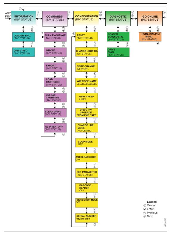
Figure 13-7 3581 2U Offline Menu - Fibre Channel drive
