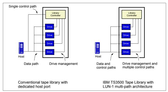
Figure 2-42 Conventional tape library versus multi-path architecture
