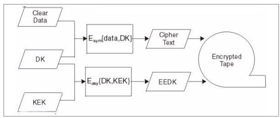
Figure 2-30 Tape Encryption process flow of the TS1120 Tape Drive
