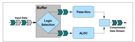
Figure 2-11 LTO-DC block diagram
