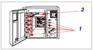
Figure 12-2 IBM 3581 cartridge slots
