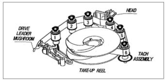
Figure 1-6 DLT tape path mechanism
