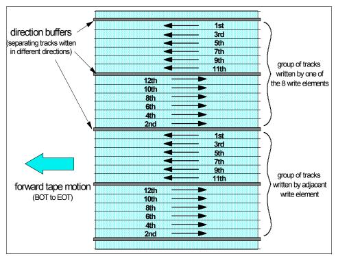
Figure 2-9 Portion of data band showing Ultrium 1 track-writing sequence
