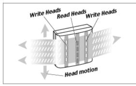
Figure 1-10 DLT 7000/8000 tape head
