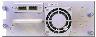
Figure 7-6 The back side of the SAS tape drive
