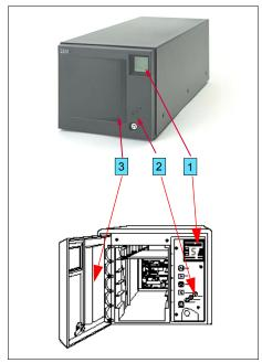
Figure 12-3 IBM 3581 front view
