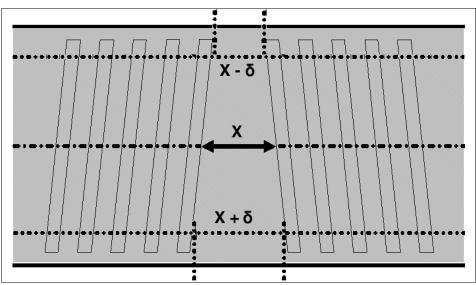
Figure 2-6 Magnified servo band showing a pair of servo bursts
