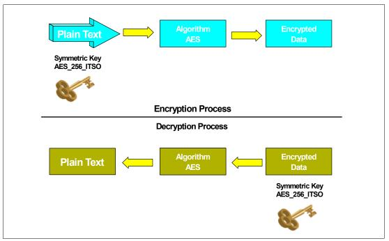
Figure 2-28 Symmetric key encryption data flow
