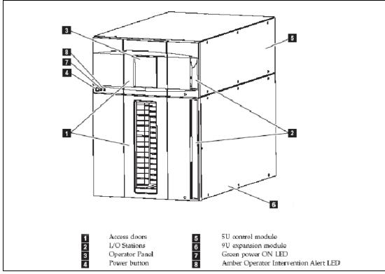
Figure 7-4 Elements visible in the front view of a 14U library configuration
