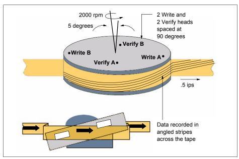
Figure 1-4 Helical-scan recording diagram
