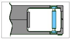
Figure 2-18 Correct leader pin placement
