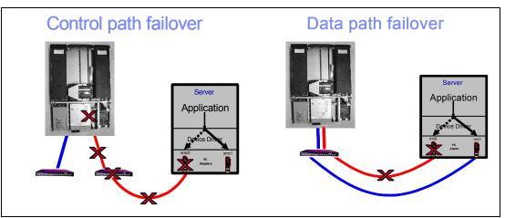
Figure 6-3 summarizes control path and data path failover with the TS3200.
