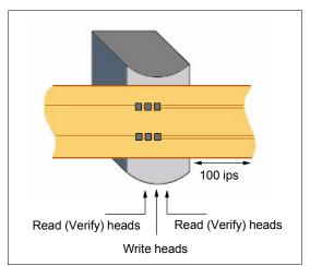
Figure 1-3 QIC head diagram
