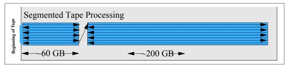
Figure 2-48 Segmented tape processing
