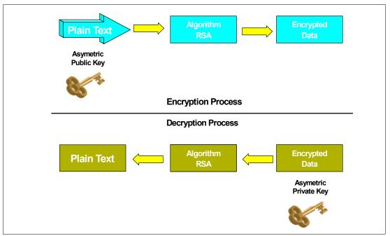
Figure 2-29 Asymmetric key encryption data flow
