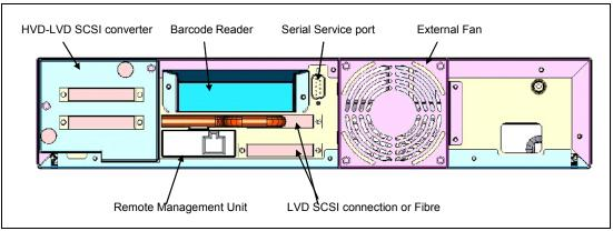
Figure 13-3 Back view of the IBM 3581 2U
