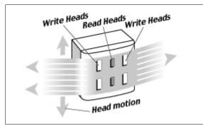
Figure 1-7 DLT 2000 recording head design
