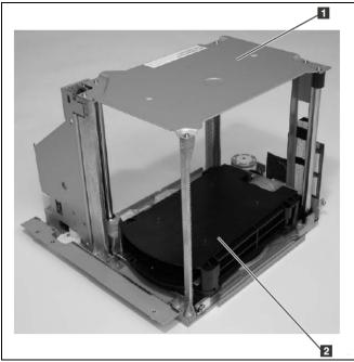
Figure 8-3 TS3400 Accessor Assembly with the picker
