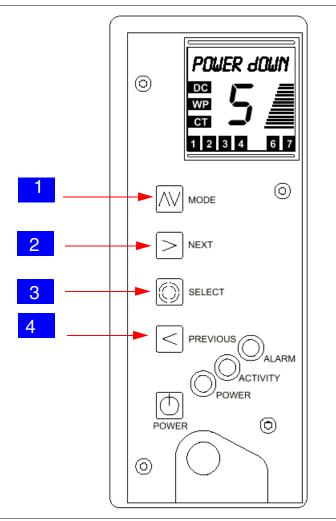
Figure 12-5 IBM 3581 Operator Panel
