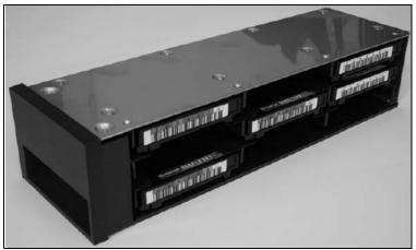
Figure 8-7 Cartridge magazine of the TS3400
