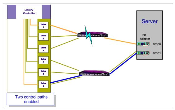
Figure 2-43 Redundant control paths to the library controller
