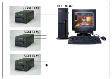
Figure 11-3 SCSI ID setup example
