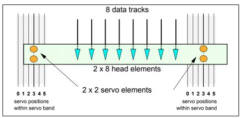
Figure 2-20 Generation 1 and 2: One of eight element heads shown, with servo elements
