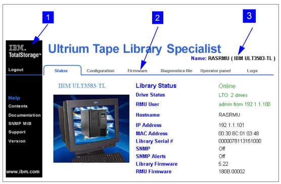
Figure 15-9 IBM 3583 TotalStorage Specialist Web interface
