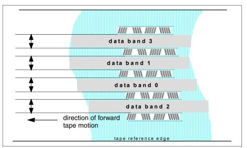
Figure 2-8 Four data bands written between the servo tracks
