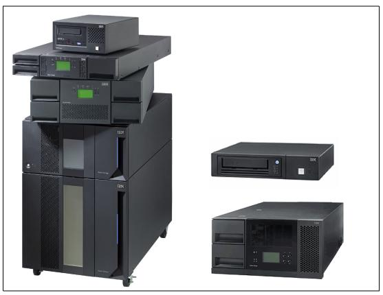
Figure 2-41 IBM 3580 Tape Drive, TS3100, TS3200, and TS3310 Tape LIbraries
