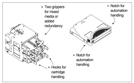
Figure 9-11 IBM TS3500 Tape Library gripper
