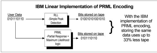
Figure 2-35 IBM linear implementation of PRML encoding
