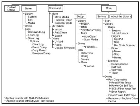
Figure 15-6 IBM 3583 flow chart of library functions
