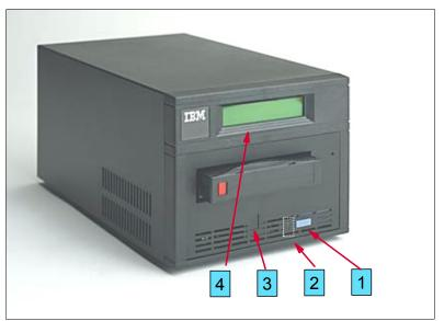
Figure 11-4 Front view of the IBM 3580 model L11/L13/L23 or H11/H13/H23 Tape Drive
