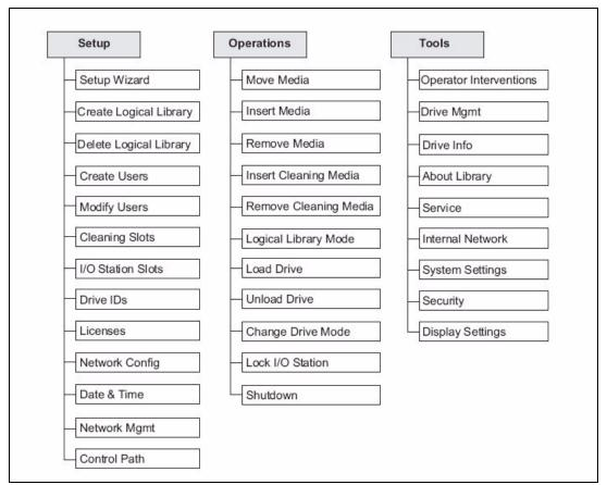
Figure 7-8 Operator Panel menu tree
