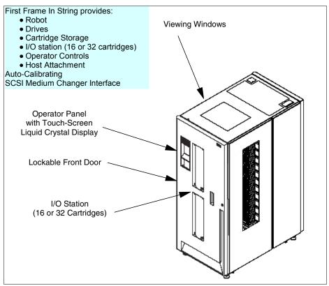
Figure 9-2 IBM TS3500 Tape Library L53 base frame view from front left
