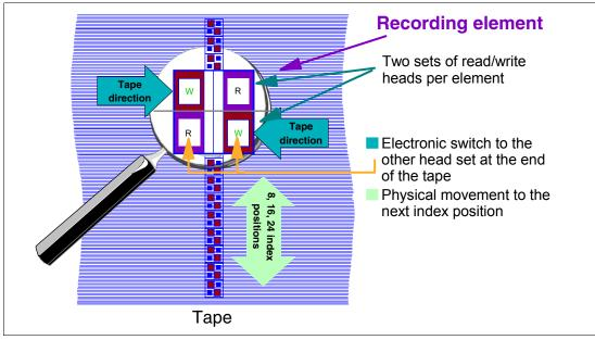
Figure 1-14 IBM 3590 recording
