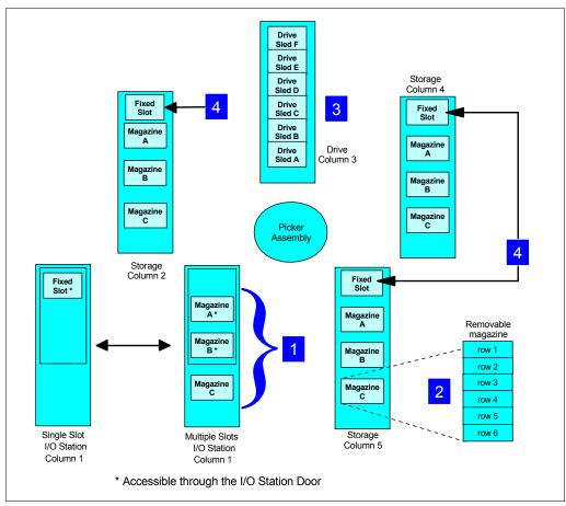
Figure 15-3 IBM 3583-L72 location logical view
