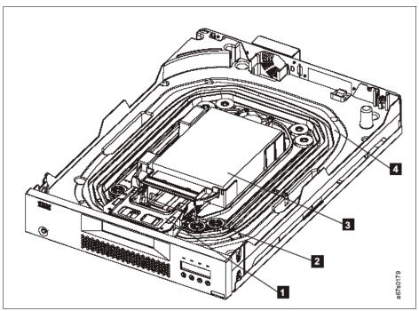
Figure 13-2 Interior components with one cartridge slot
