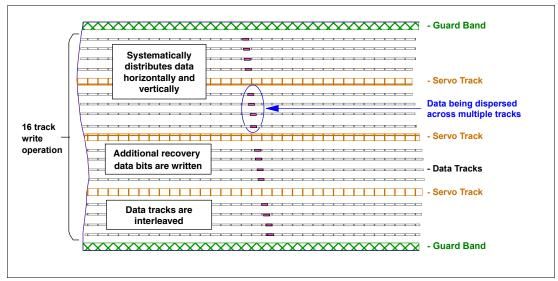
Figure 1-15 IBM TotalStorage 3590 tape data integrity
