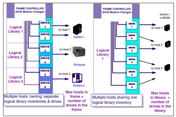
Figure 1-19 IBM 3584 multi-path architecture
