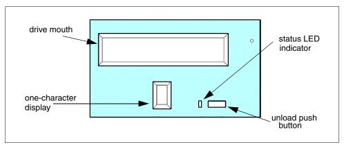
Figure 2-36 Front of subassembly showing Operator Panel indicators
