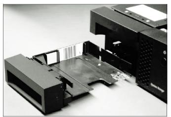
Figure 5-8 I/O station in the left magazine
