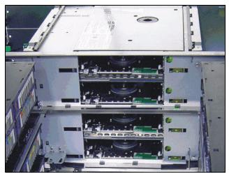
Figure 6-6 Interior of the TS3200 with four Ultrium 3 Half-High drives installed
