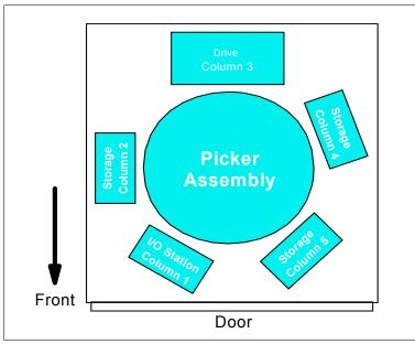
Figure 15-2 IBM 3583 storage columns: Top view
