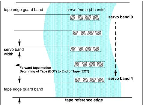
Figure 2-5 Servo band position and nomenclature
