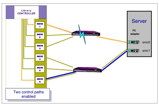
Figure 9-13 Redundant control paths to the library controller
