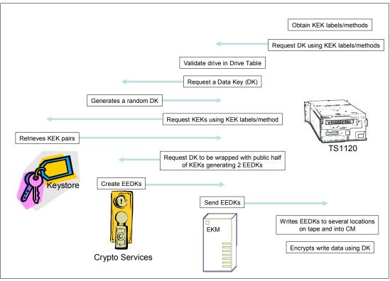
Figure 2-31 Encryption process TS1120
