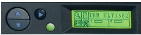
Figure 14-4 IBM 3582 Operator Panel
