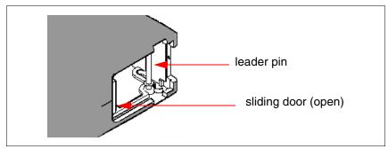
Figure 2-14 Leader pin attached to the tape medium
