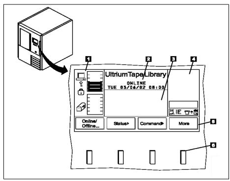
Figure 15-5 IBM 3583 Operator Panel
