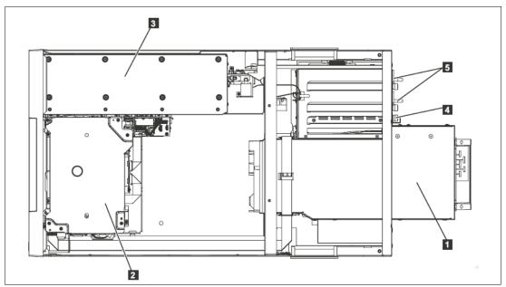
Figure 8-2 Interior components of the IBM System Storage TS3400 Tape Library
