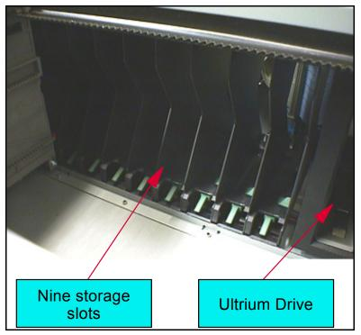
Figure 14-3 IBM 3582 rear-mounted storage slots
