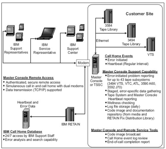
Figure 9-14 Flow of data from a Master Console supporting three Tape Libraries
