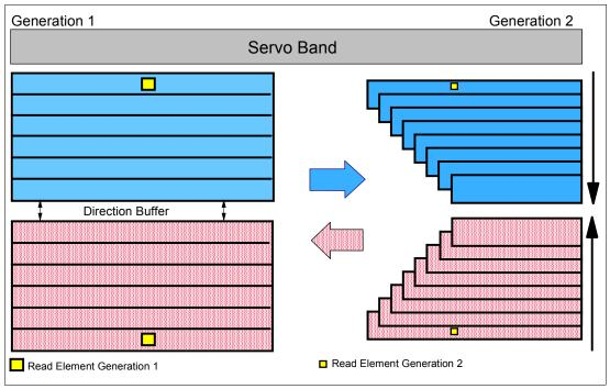
Figure 2-10 Shingling: Writing to tape generation 1 versus generation 2
