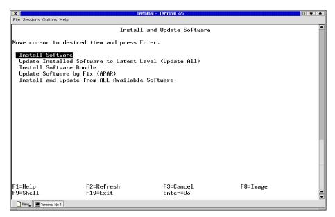
Figure 2-4 SMIT installp window (ASCII or text-based interface)
