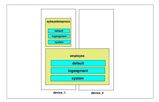
Figure 5. Segments on device\_1 and device\_2
