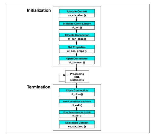
Figure 42 shows the function call sequences for initialization and termination.
