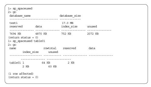
Figure 17. sp\_spaceused stored procedure
