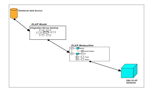
Figure 42. Integration Server to DB2 OLAP flow illustration
