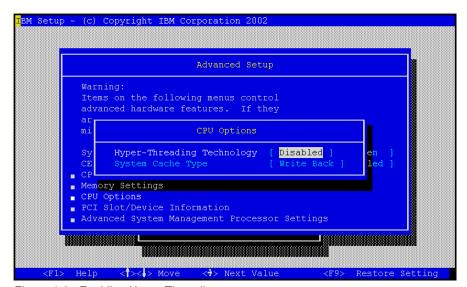
Figure 4-2 Enabling Hyper-Threading
