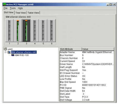
Figure 5-12 IBM Gigabit Ethernet Adapter installed in slot 3
