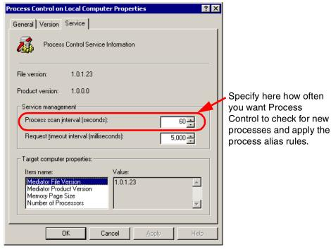
Figure 5-45 Process Control scan interval
