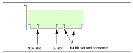
Figure 5-14 The meaning of the slots in the PCI connector
