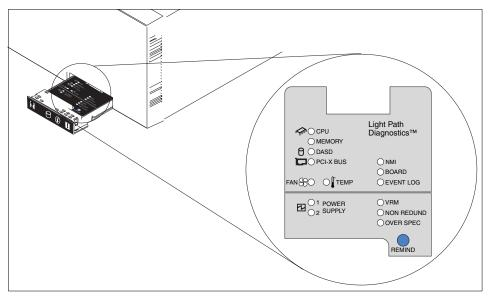
Figure 1-14 Light Path Diagnostics panel on the x440
