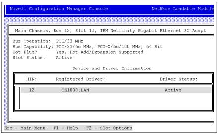
Figure 4-13 Shows that hot-plug is enabled
