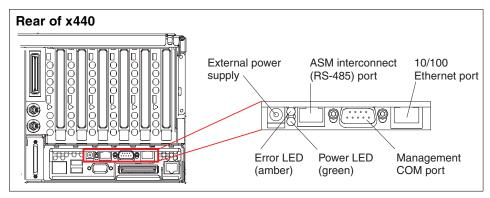
Figure 1-15 Remote Supervisor Adapter connectors
