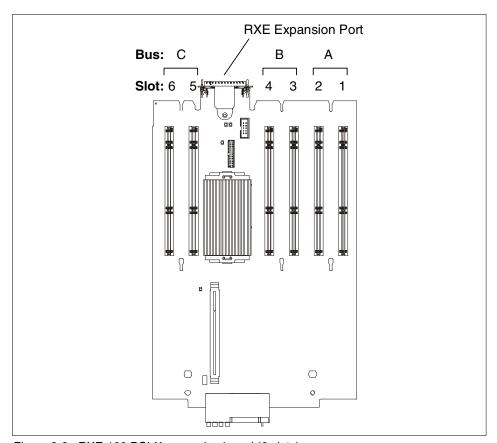
Figure 3-8 RXE-100 PCI-X expansion board (6 slots)
