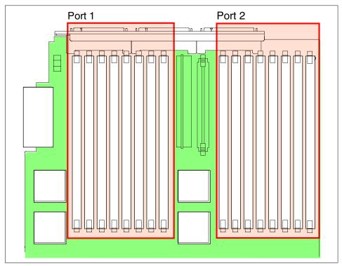
Figure 1-12 Memory DIMMs are divided into two ports
