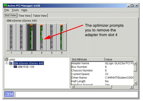
Figure 5-18 Removing an adapter from slot 4
