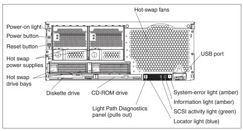
Figure 1-13 Front panel of the xSeries 440
