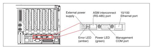
Figure 3-7 Remote Supervisor Adapter Connectors
