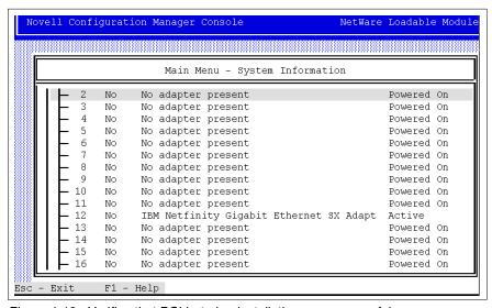
Figure 4-12 Verifies that PCI hot-plug installation was successful
