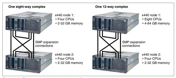
Figure 1-3 Eight-way and 12-way two-node configurations
