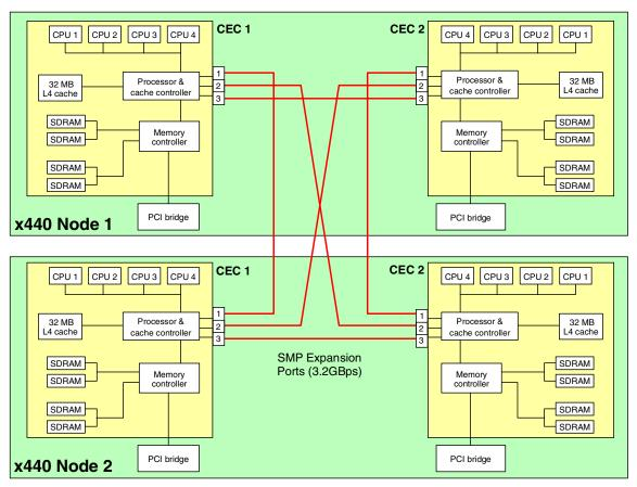
Figure 1-6 16-way configuration (four SMP Expansion Modules)
