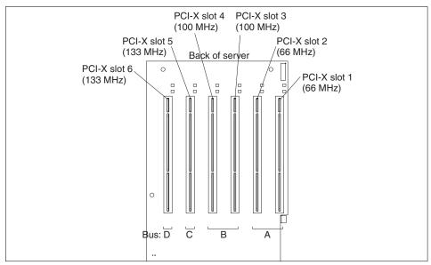
Figure 3-3 PCI-X slots in the x440
