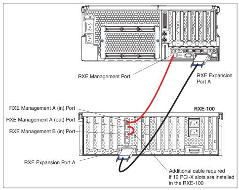
Figure 3-9 Connecting the RXE-100 to the x440
