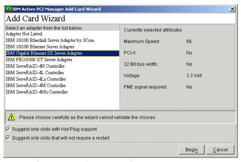
Figure 5-8 Selecting the IBM Gigabit Ethernet SX Adapter
