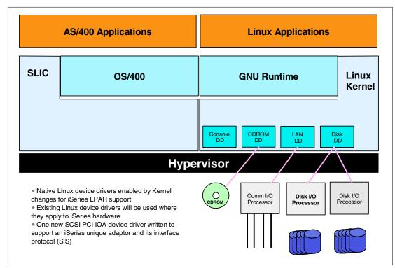
Figure 1-3 Direct attached IOA
