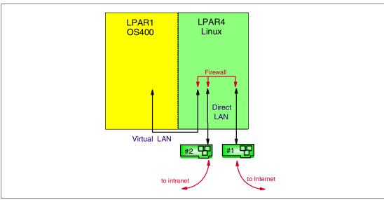
Figure 8-7 A firewall without perimeter network
