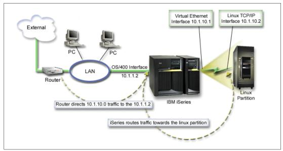
Figure 2-44 TCP/IP routing example
