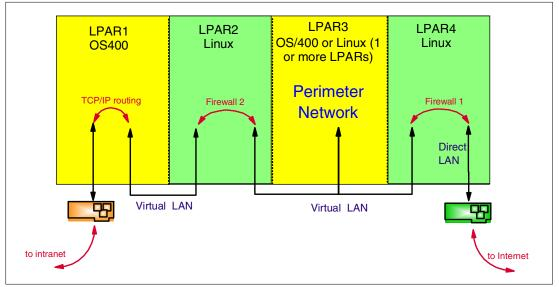
Figure 8-3 A basic configuration with a perimeter network
