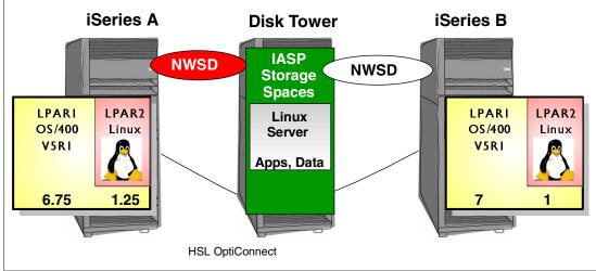
Figure A-3 Example of a Linux NWSSTG on an Independent ASP
