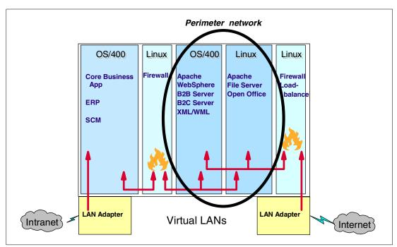
Figure 1-4 Scenario using Linux partitions to create a perimeter network (DMZ)
