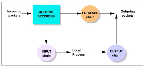
Figure 8-1 INPUT and FORWARD and OUTPUT chains
