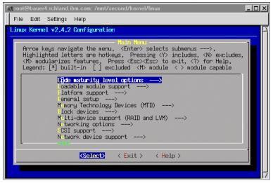
Figure 4-1 Configuring the kernel using make menuconfig
