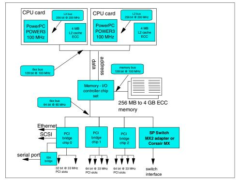
Figure 2-3 POWER3 SMP system architecture
