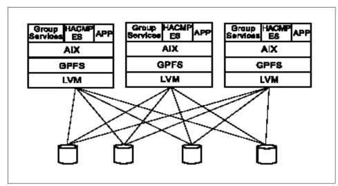
Figure 8-2 A GPFS configuration for an HACMP cluster environment
