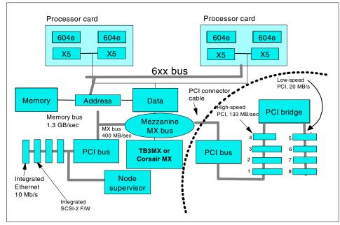
Figure 2-2 PowerPC 604e 332 MHz processor
