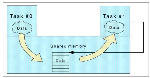
Figure 6-2 Intranode communication with shared memory segment
