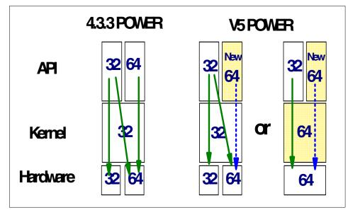
Figure 3-1 AIX 5L Version 5.1- New 64 bit Kernel and API
