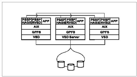
Figure 8-1 A GPFS configuration in an SP environment
