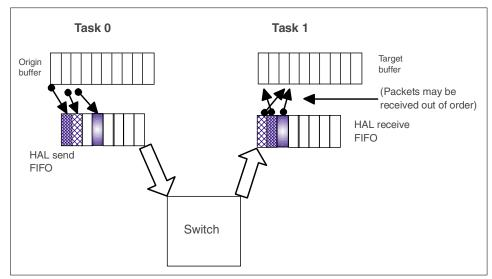
Figure 6-1 Intranode communication with switch
