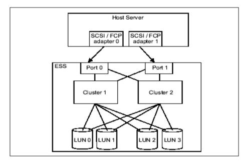
Figure 3-2 ESS disk configuration with multipath connections to a host system
