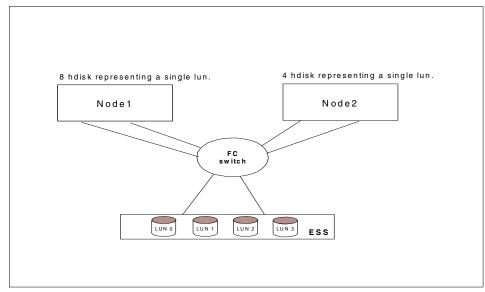
Figure 3-3 Fibre Channel switch configuration: two hosts connecting to an ESS
