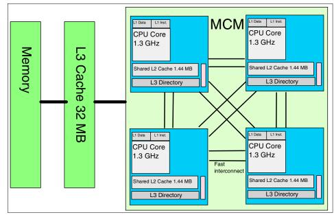
Figure 2-5 Simplified layout of a High Performance Computing MCM
