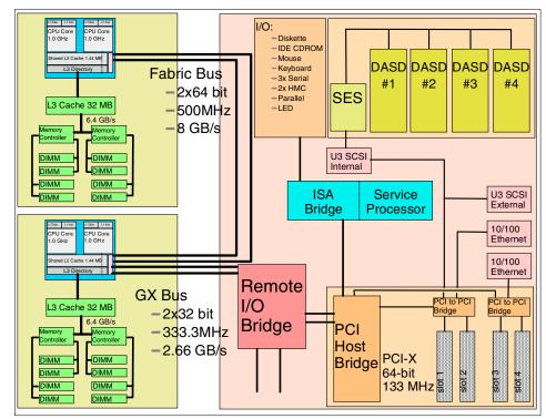
Figure 2-3 Design layout of the p630
