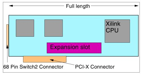
Figure 2-15 Layout of the SP Switch2 PCI-X Attachment Adapter (FC 8398)
