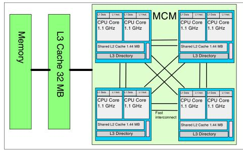
Figure 2-9 Simplified layout of an MCM as installed in a p670 (8-way)
