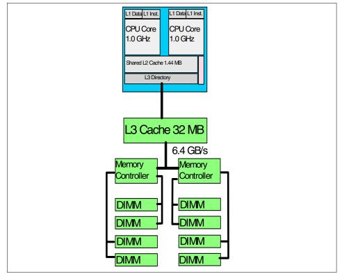
Figure 2-2 Design of the CPU board of the p630 with a POWER4 SCM
