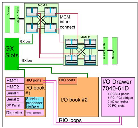
Figure 2-10 Simplified diagram of the p670 interconnection
