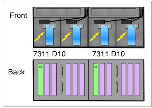
Figure 2-18 Two 7311 D10 I/O drawers side by side
