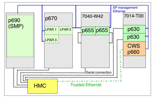
Figure 6-3 Connection between the HMC and the CWS
