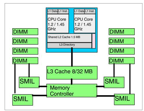
Figure 2-11 Simplified layout of a p650 processor card
