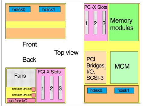
Figure 2-7 Simplified layout of the p655
