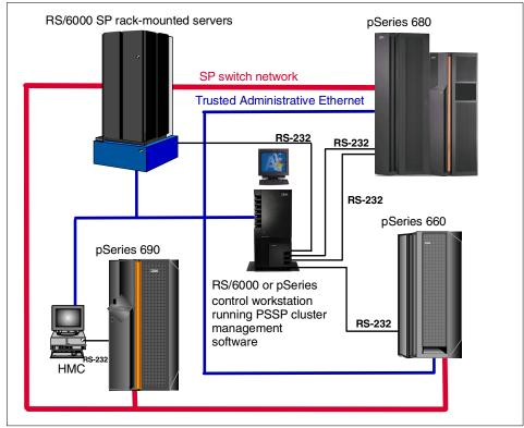
Figure 1-1 Example of an IBM eServer Cluster 1600 managed by PSSP
