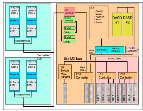
Figure 2-14 System layout of an SP Winterhawk-II wide node
