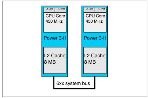
Figure 2-13 A two processor card in a Winterhawk-II SP node
