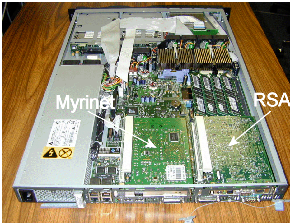
Figure 3-1 x330 with PCI cards installed
