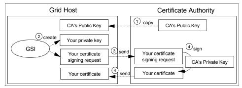
Figure 3-3 Preparation procedure for GSI
