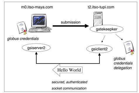
Figure 7-3 Using globus\_io for secure communication
