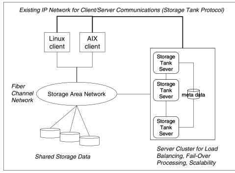
Figure 4-10 Storage Tank architecture
