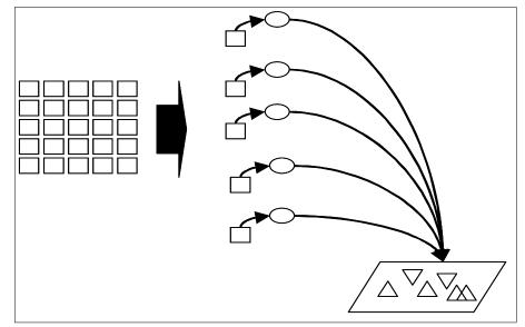
Figure 4-6 Jobs with individual input data writing output into one data store
