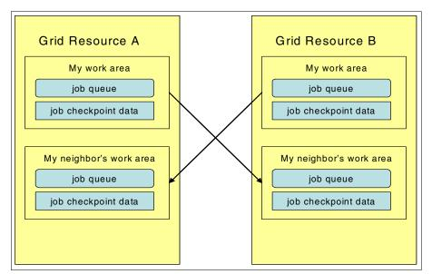
Figure 2-4 Share job information for fault-tolerance
