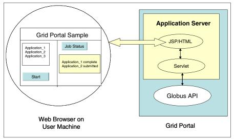
Figure 2-5 Grid portal on an application server
