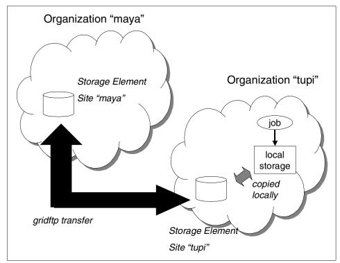
Figure 4-12 File replication in a data grid between two organizations
