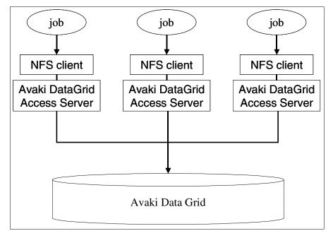
Figure 4-8 Accessing Avaki Data Grid through NFS locally mounted file system
