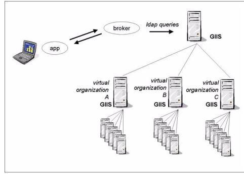
Figure 5-3 Working with a broker
