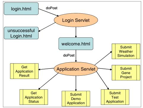
Figure 8-3 Simple grid portal application flow
